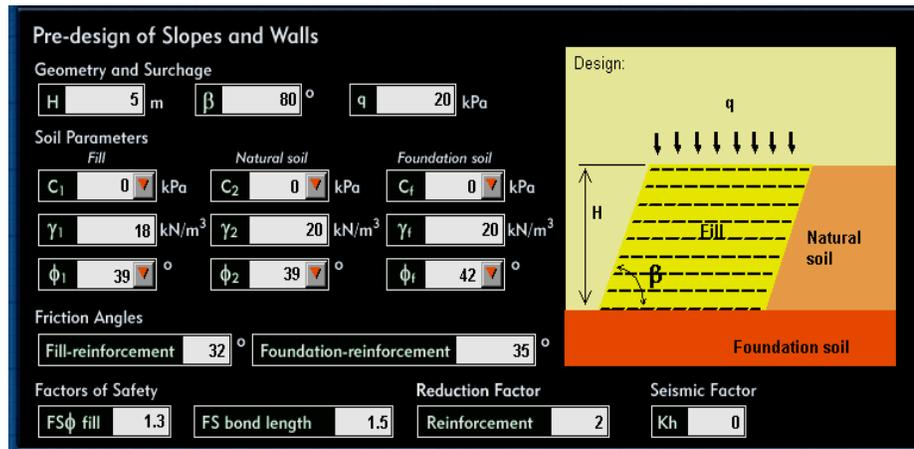
Fig.20 The Slope with Geometric Properties ( $\beta= 80^\circ$ ).
