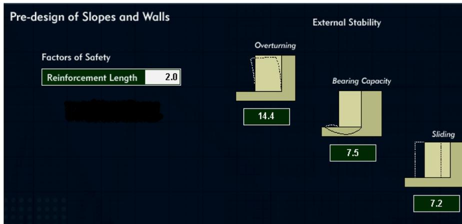
Fig.28 The Slope Factors of Safety.
