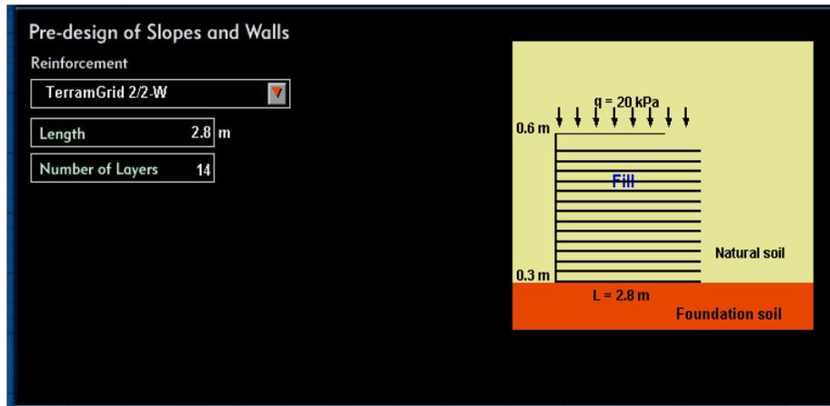
Fig.18 The Slope after Reinforcement.
