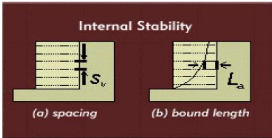
Fig.1 Internal Stability of the Wall.
