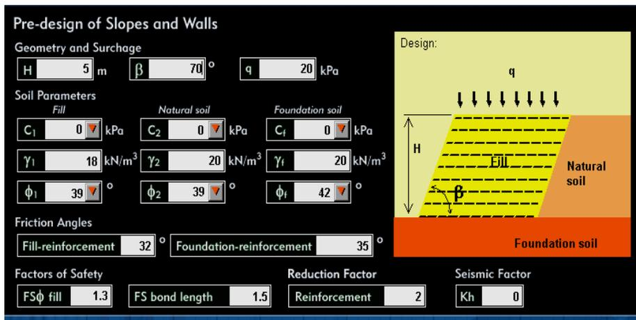
Fig.23 The Slope with Geometric Properties ( $\beta= 70^\circ$ ).
