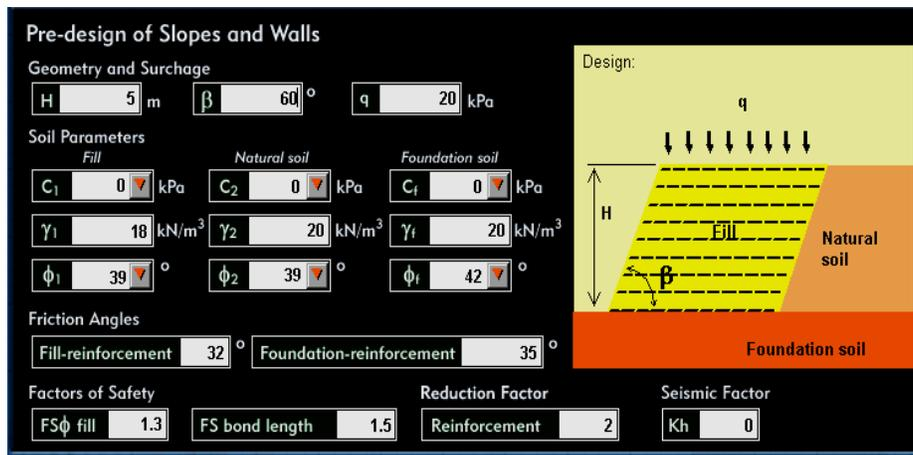
**Fig.26 The Slope with Geometric Properties ( $\beta= 60^\circ$ ).**
