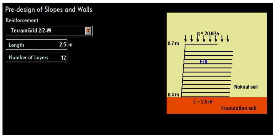
Fig.21: The Slope after Reinforcement.
