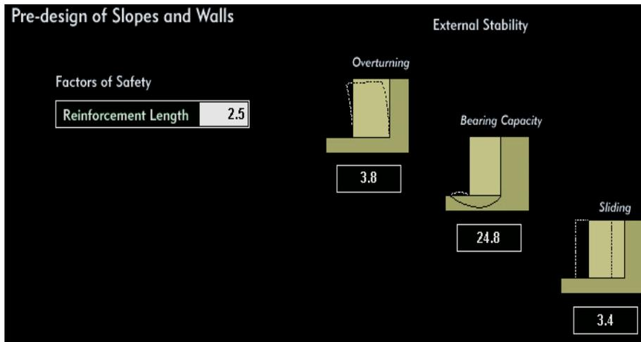
**Fig.7 The Wall Factors of Safety.**
