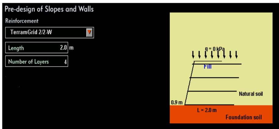
Fig.15 The Slope after Reinforcement.
