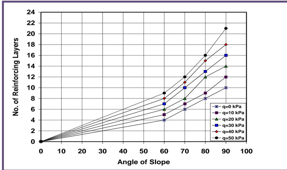
**Fig.29 No. of Reinforcing Layers versus Angle of Slope for different q with H= 5m.**
