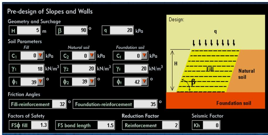
**Fig.17 The Slope with Geometric Properties ( $\beta= 90^\circ$ ).**
