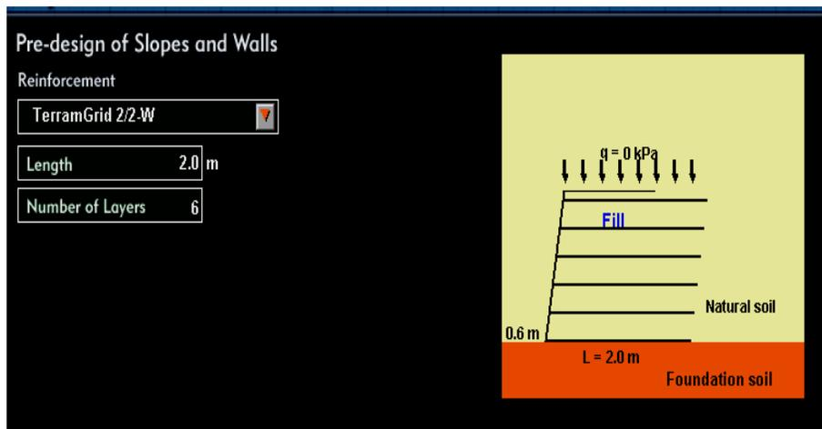
**Fig.12 The Slope after Reinforcement.**
