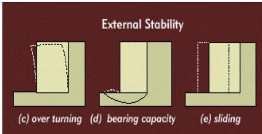
Fig.2 External Stability of the Wall.
