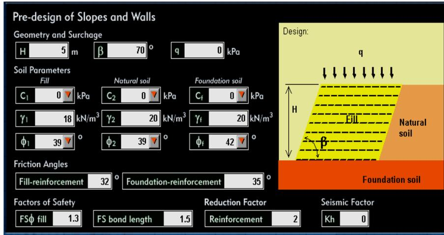
**Fig.11 The Slope with Geometric Properties ( $\beta= 70^\circ$ ).**
