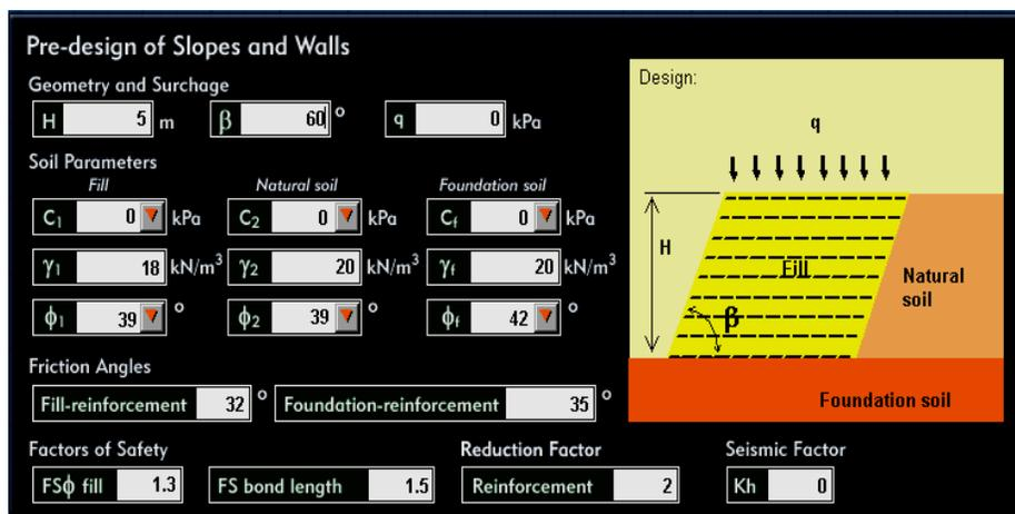
Fig.14 The Slope with Geometric Properties ( $\beta= 60^\circ$ ).
