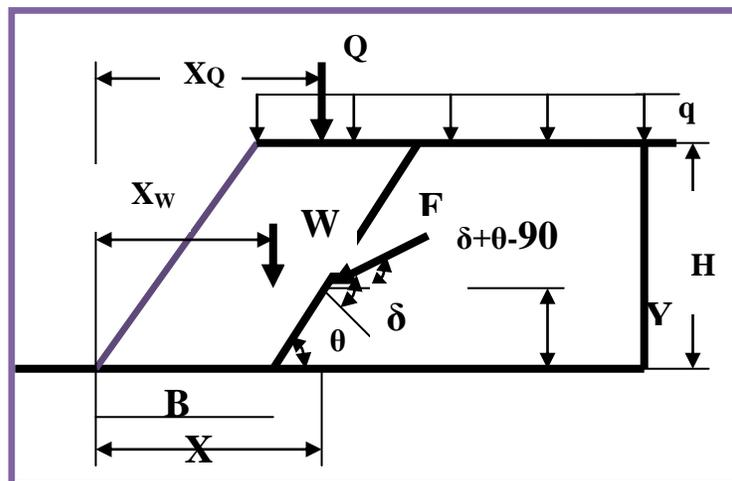
Fig.3 The Overturning Stability.
