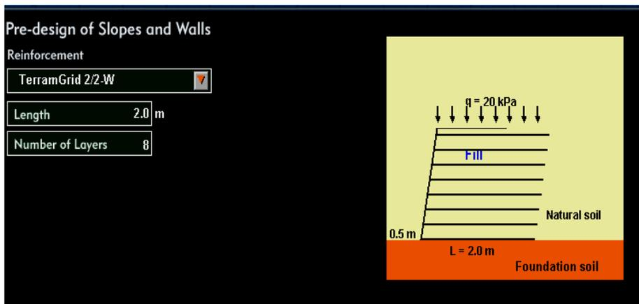
Fig.24 The Slope after Reinforcement.
