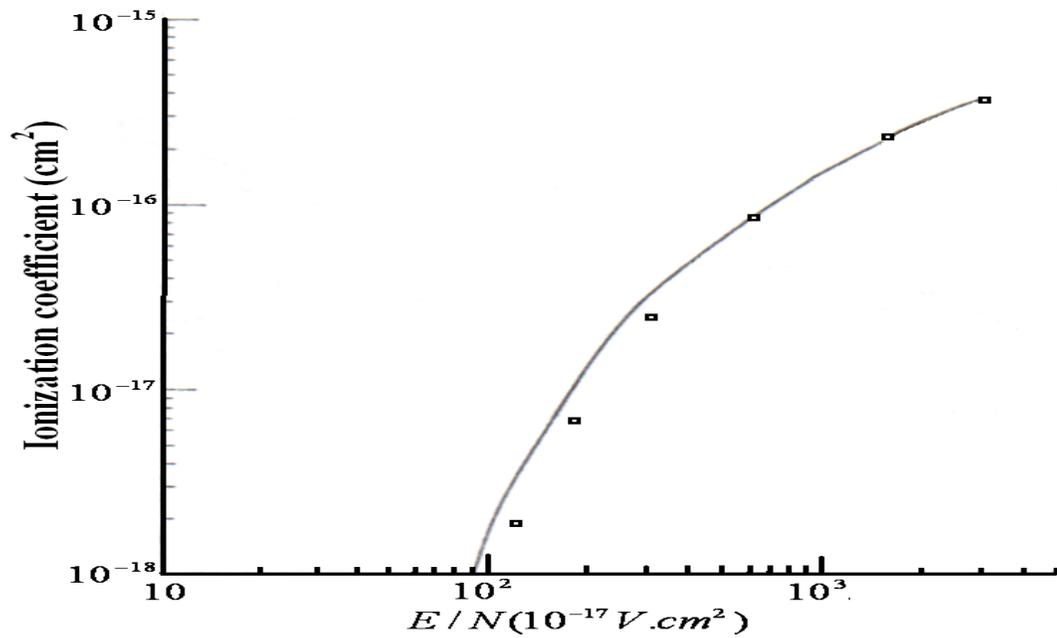
Figure 8: The ionization coefficient of electrons as a function for  $E/N$  in Carbon Dioxide.
