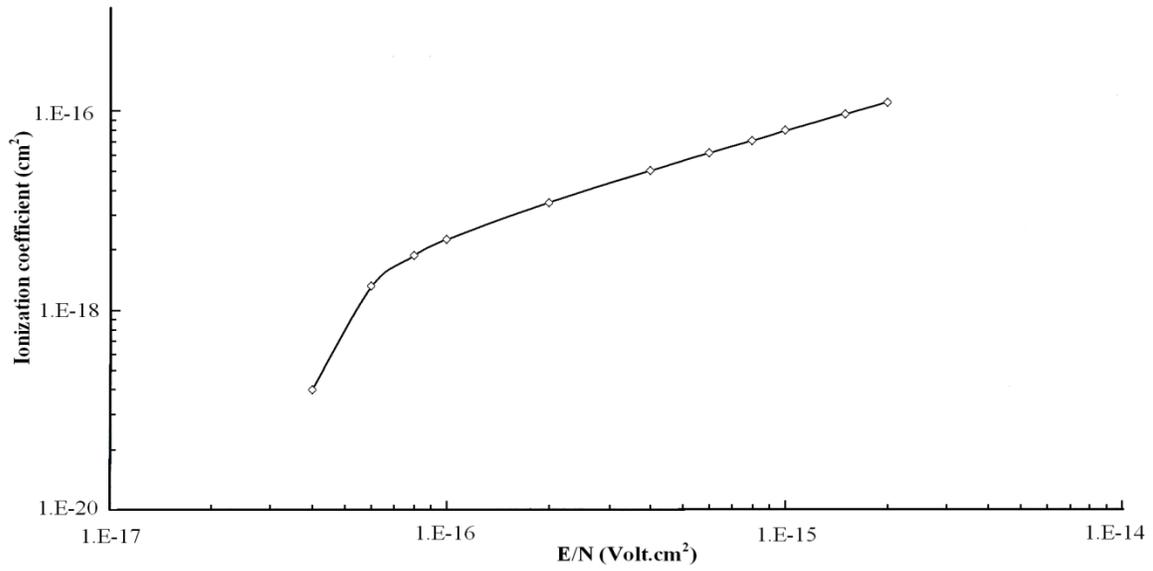
Figure 7: The ionization coefficient of electrons as a function of  $E/N$  for pure Xenon gas.
