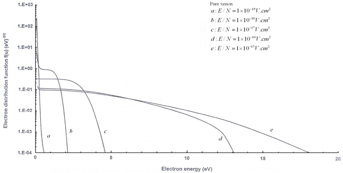
Figure 1: The electron energy distribution function in pure xenon gas for several values of  $E/N$ .
