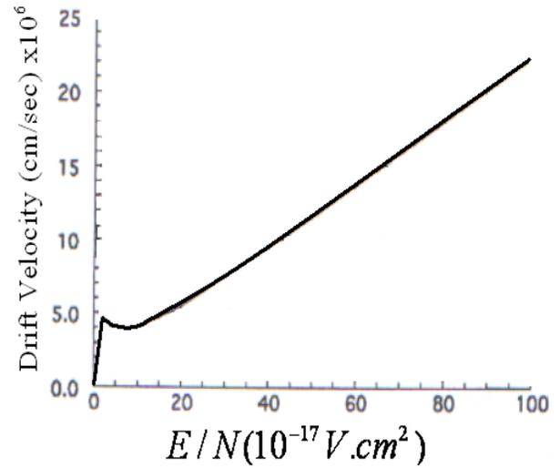
Figure 6: The drift velocity as a function of  $E/N$  for  $\text{CO}_2\text{-Xe}$  (10:90).
