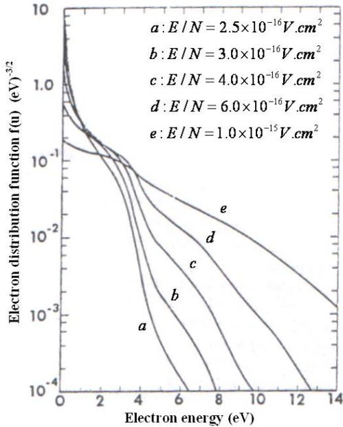
Figure 2: The electron energy distribution function in pure Carbon dioxide as a function of  $E/N$  for several values of  $E/N$ .
