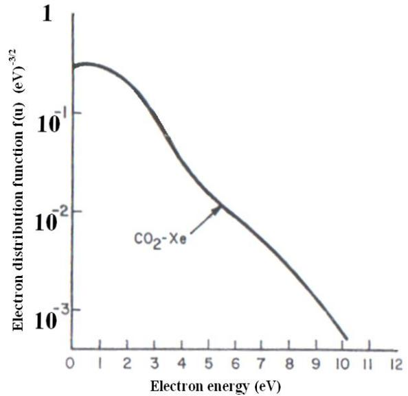
Figure 3: The electron energy distribution function as a function of electron energy in  $CO_2:Xe$  gas mixtures (50:50) at  $E/N = 3 \times 10^{-16} V.cm^2$ .
