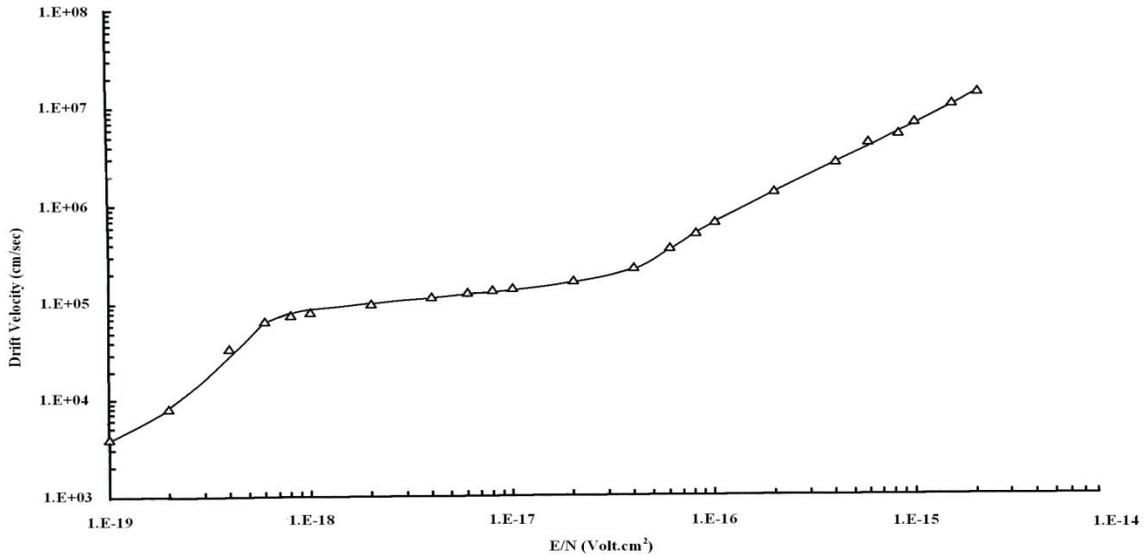
Figure 4: The drift velocity of electron as a function of  $E/N$  for pure xenon gas.
