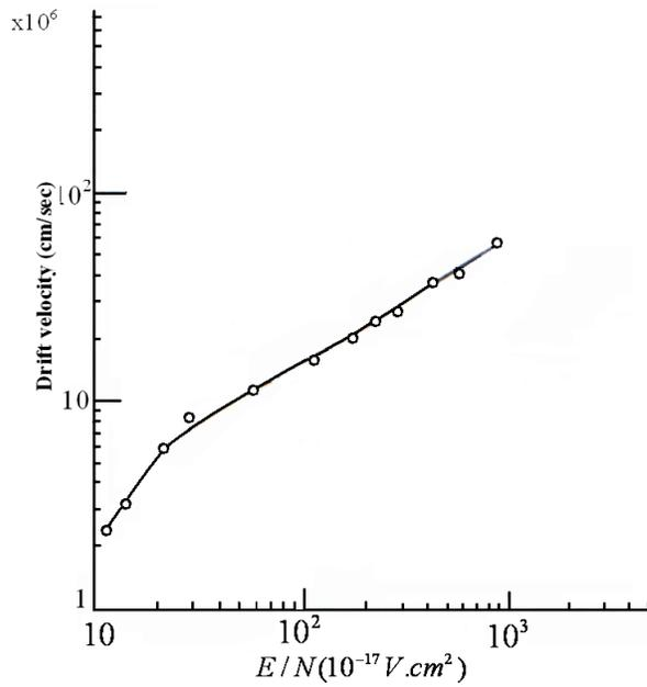
Figure 5: The drift velocity as a function of  $E/N$  for Carbon dioxide.
