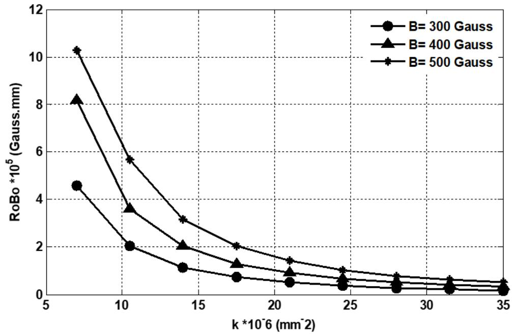
**Fig. 1:** The magnetic rigidity versus focusing strength factor with different magnetic field
