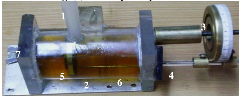
Fig. (2) Device of studying of the breakdown phenomena: (1) vent to pressure balance; (2) pin electrode; (3) micrometer; (4) glass tube; (5) plane electrode; (6) body of cell; (7) support cell; and (8) base of device.
