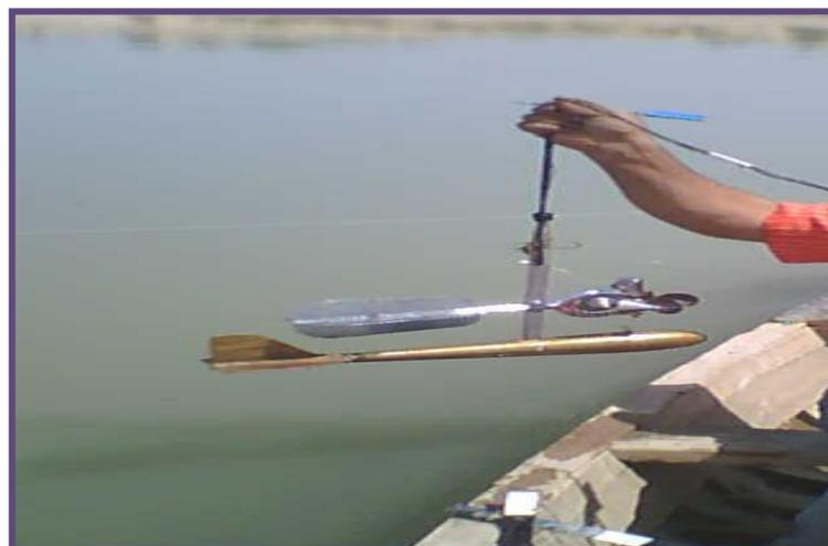
**Fig. 8 : The Current Meter in this Study.**
