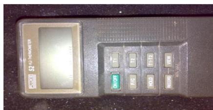
**Figure (3-b) Thermometers Types k/j**
