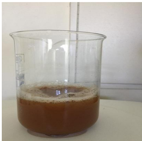
Figure 3- Samples after a prank of distilled water and put it on the fire for one hour and at a temperature of moderate 60 degrees
