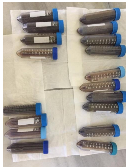
Figure 6- Models of nanoparticles extracted with plant extracts for the purpose of isolating the material by centrifugation
