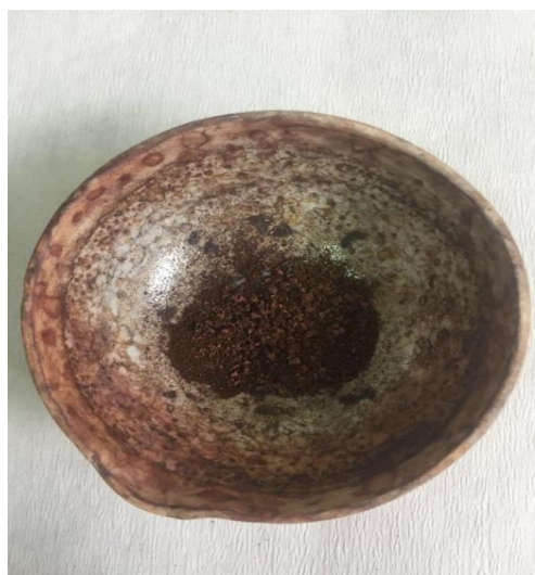
Figure 5- nanoparticles produced after being placed in the oven under 400 degrees heating
