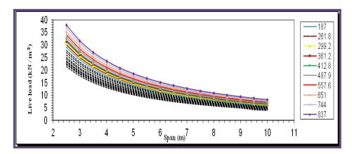
Fig.13 Live Load- Span Relation due to Shear Condition (with Topping).
