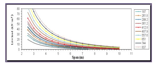
Fig.12 Live Load- Span Relation due to Flexural Condition (with Topping).
