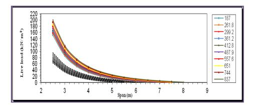
Fig.14 Live Load-Span Relation due to Deflection Condition (with Topping).
