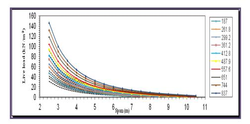
Fig.15 Live Load- Span Relation due to Allowable Stress Condition (with Topping).
