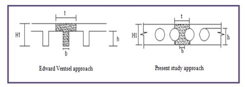
Fig.3 Equivalent Plate of Hollow Core Slab.
