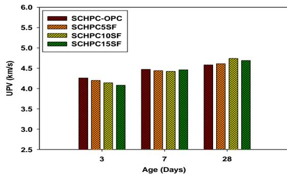
Figure 8: UPV values of SCHPC containing silica fume with age
