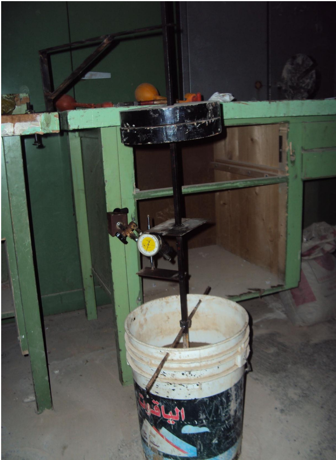
Fig. (1) : Loading frame and settlement control
