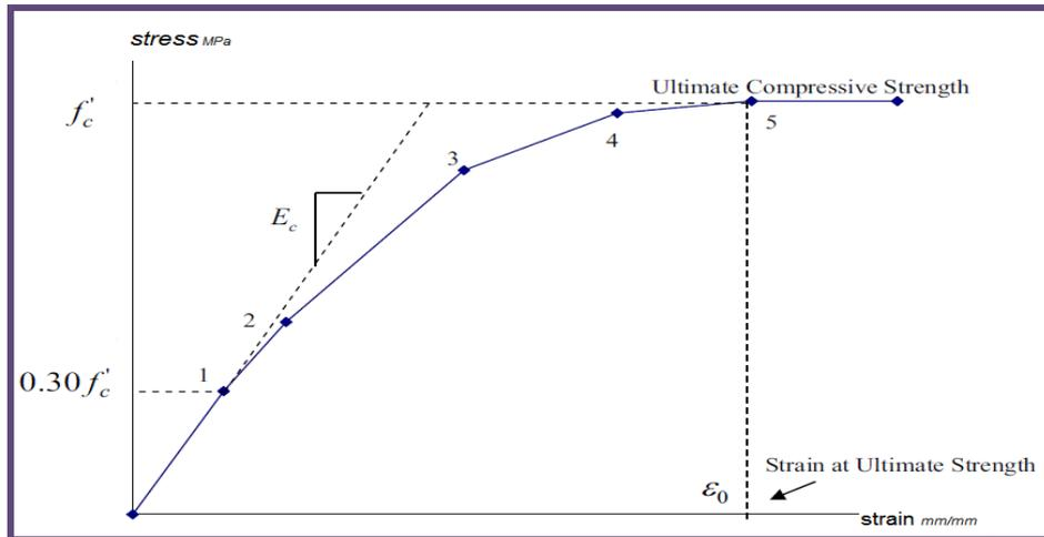
**Fig. 4 Uniaxial Stress-Strain Curve.**
