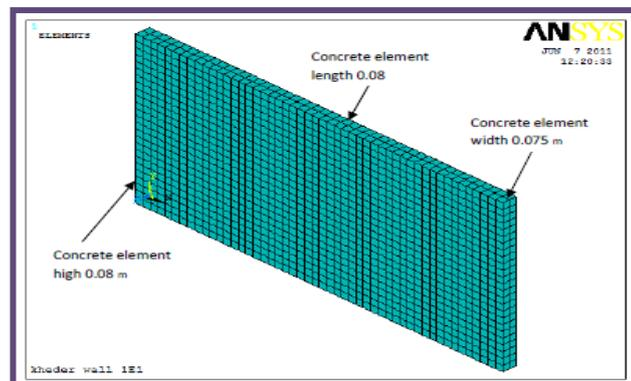
**Fig.7 Mesh of Concrete.**
