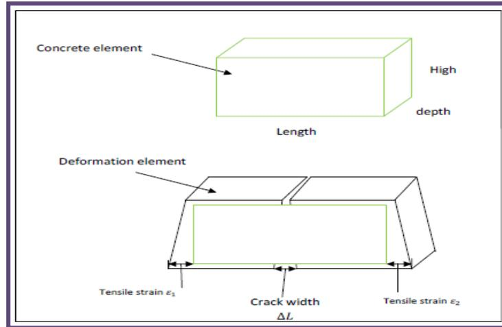
**Fig.10:Method Calculated of Crack Width.**
