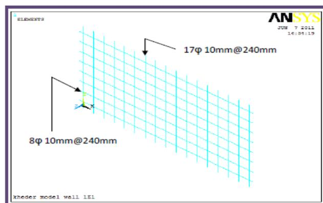
**Fig.8 Modeling of Steel Reinforcement.**
