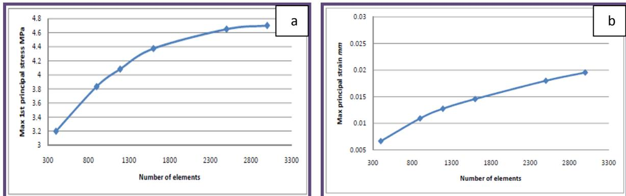
**Fig.6 (a) Maximum Principal Stresses , (b) Strains of Concrete wall.**
