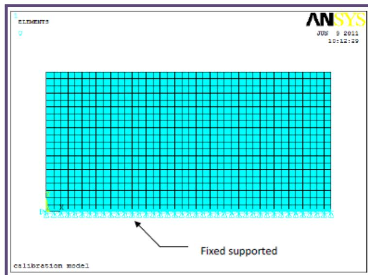
**Fig.9 Boundary Condition for Supported.**
