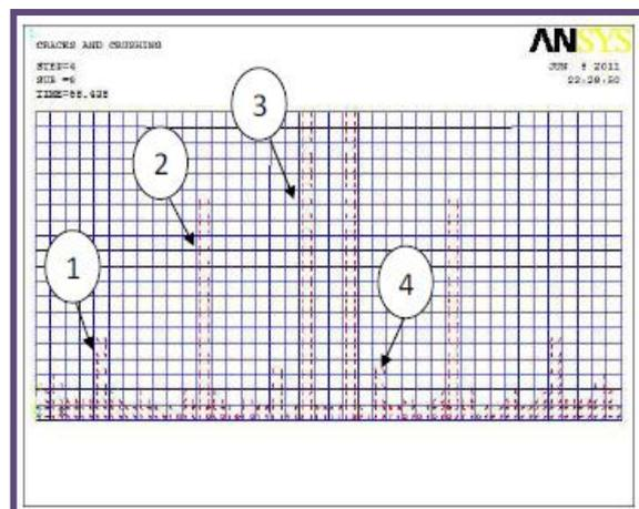
**Fig.11: Location and Numbers Cracks.**
