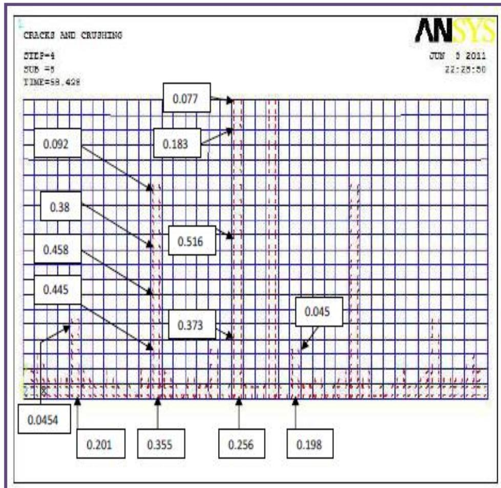
Fig.12 Crack Width for ANSYS.
