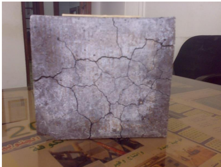
Fig 4: Spider cracks due to bad storage
