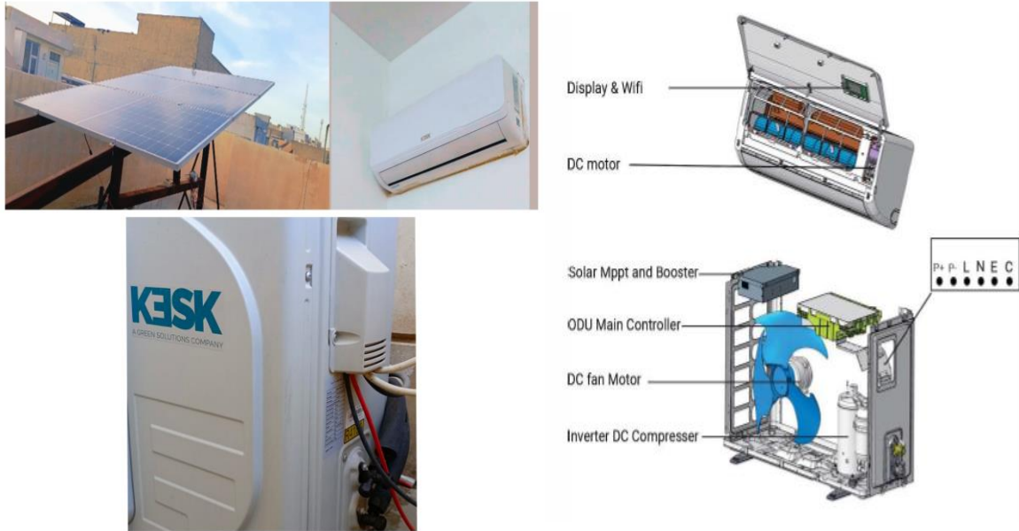
Fig 4. The photovoltaic system used in the experiment.
