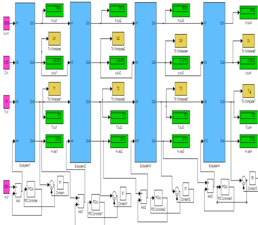
**Fig. 12** PID control for each one of the evaporators in the caustic soda system.
