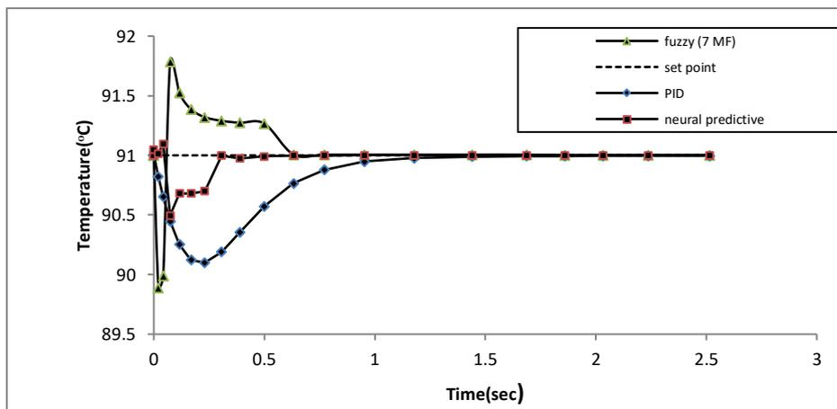
**Fig. 24** Comparing PID, NN (predictive), and fuzzy logic (7 MFs functions) in 1st evaporator to step-changes in flow rates of the feed between 10,000 & 11,000kg/hr at 91°C set point for the caustic system of the soda.
