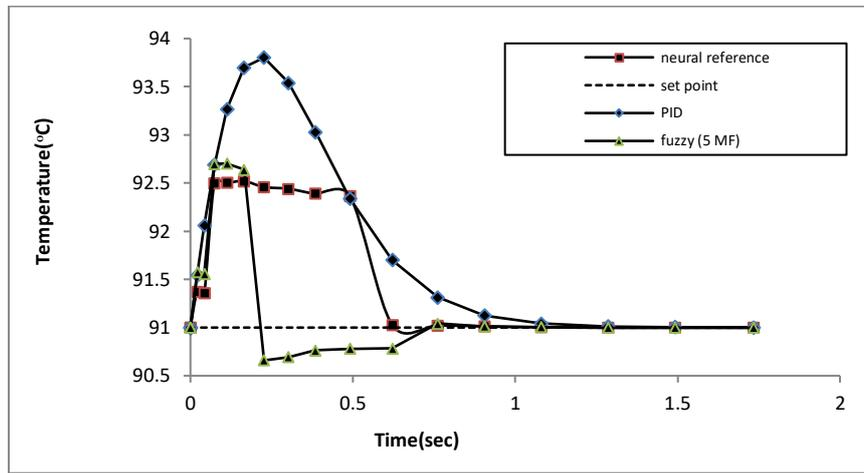
**Fig. 25** Comparing between NN (reference), PID, and fuzzy logic (5 MFs) in the 1st evaporator to step-changes in the feed temperature between 75°C – 85°C at 91°C set point for caustic soda system.
