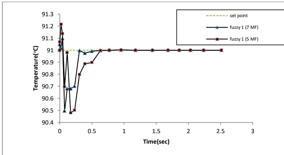
**Fig. 18** responses of Temperature that are related to 1st evaporator under 5 & 7 MFs fuzzy logic controller to the step-changes feed flow rates between 10,000 and 11,000kg/hr. at the set point =91°C.
