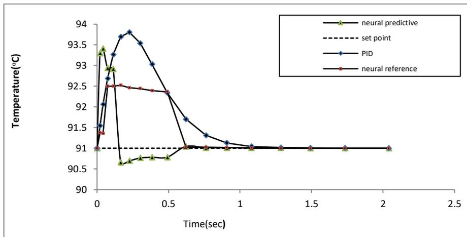
**Fig. 23** Comparing PID and neural network (predictive and reference) controllers 1st evaporator to step-changes in the feed temperature from 75°C to 85°C at a setpoint value of 91°C in the case of the caustic soda systems.
