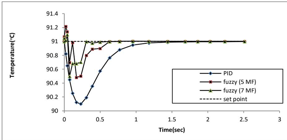
**Fig. 22** Comparing PIDs with the fuzzy logic (5 & 7 MFs) controllers in 1st evaporator to the step-changes in the flow rates of the feeds between 10,000 and 11,000kg/hr. at 91°C set point for the caustic system of the soda.
