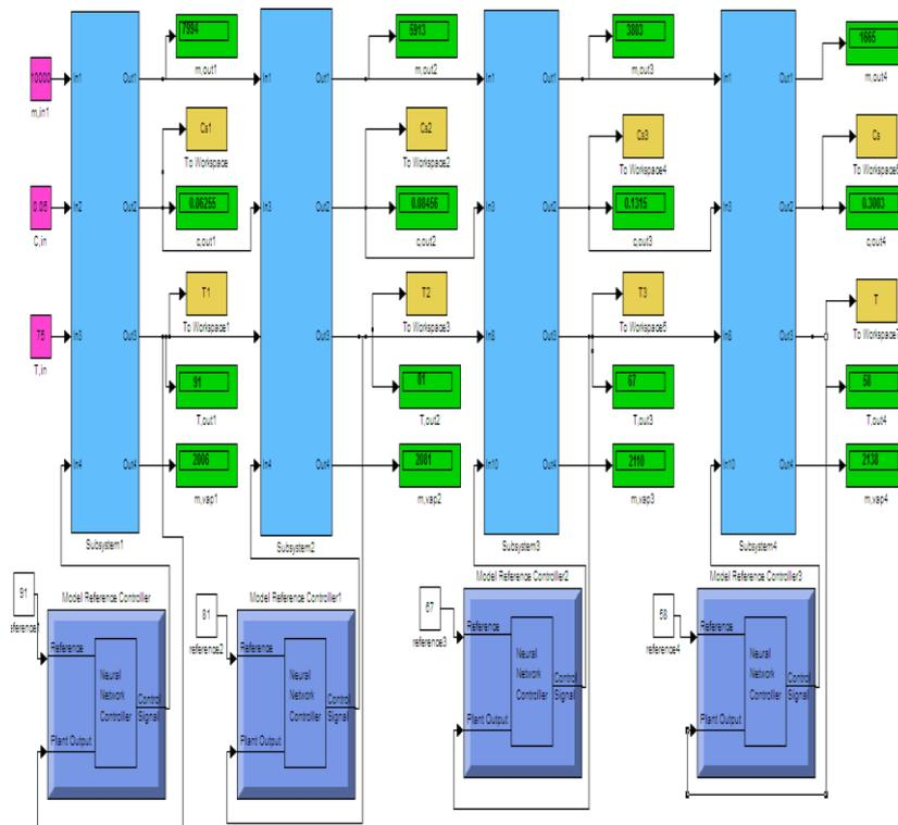
**Fig. 10** Neural Model Reference Control for caustic soda system.
