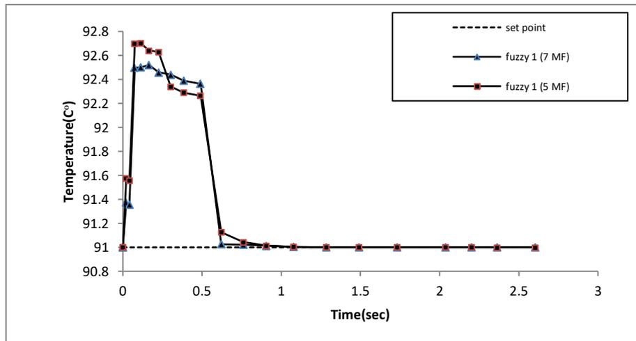
**Fig.19** responses of Temperature that are associated with the 1st evaporator under 5 & 7 MFs fuzzy logic controllers to the step changes in the temperatures of the feed between 75°C – 85°C at the set point =86°C.
