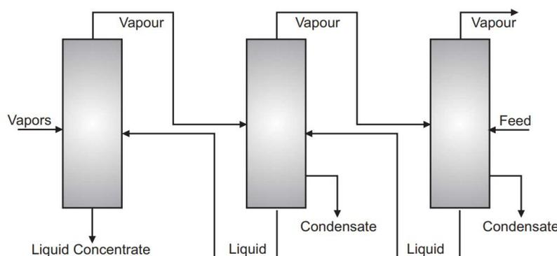
**Fig. 1** Multiple-effect evaporation equipment.
