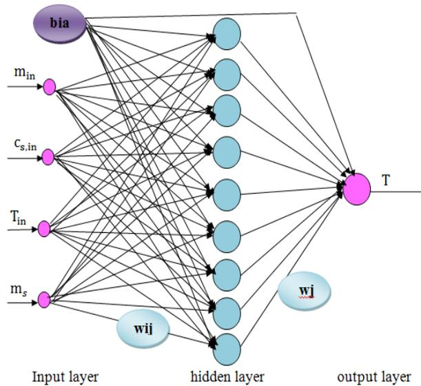
**Fig. 3 The structure of NN for the evaporator.**
