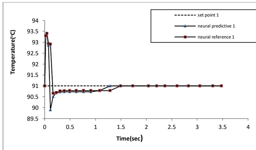
**Fig. 21** responses of the Temperature that are related to 1st evaporator under the neural predictive and neural reference controllers to the step-changes in the feed temperatures between 75°C – 85°C at 91°C set point.
