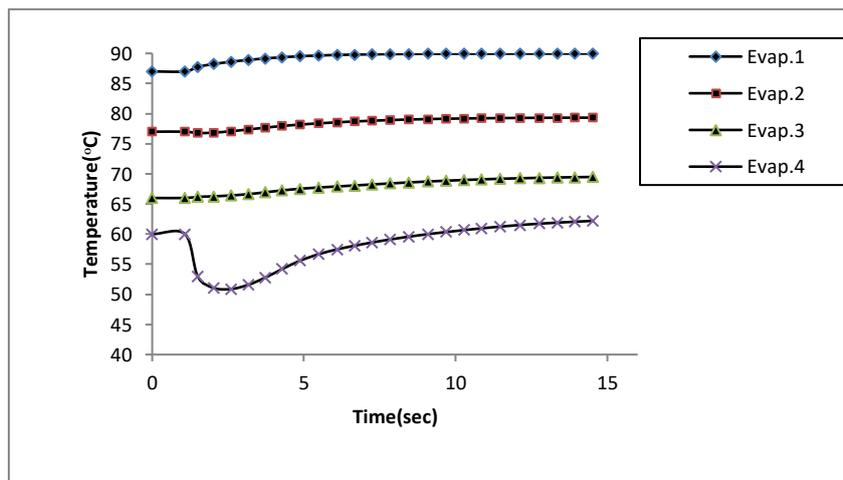
**Fig. (16)** The evaporators of the temperature response to the step changes in concentration feed between 0.05 and 0.06 kg solid/kg solution.
