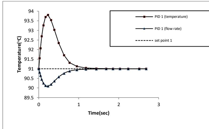
**Fig. 17** responses of temperature of 1st evaporator for the PID controller to a step-change in feed flow rates between 10,000 and 11,000kg/hr and step changes in feed temperatures between 75°C and 85°C at set point which is equal to 91°C.
