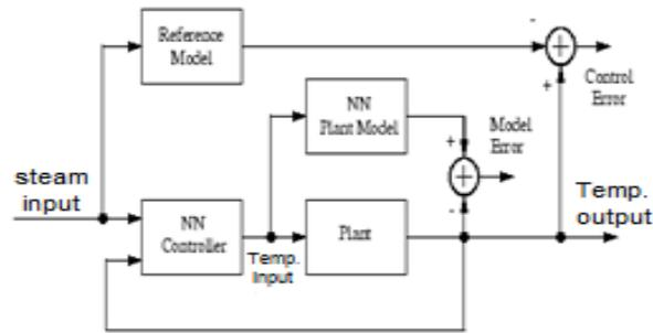
**Fig. 4** A typical Reference Control system.
