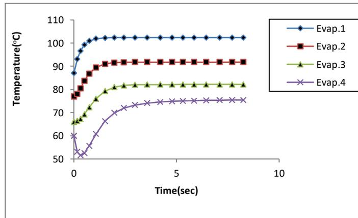
**Fig. 13** Evaporators' temperature response to the step-changes in flow rates of the steam between 2,381 and 2,619kg/hr.
