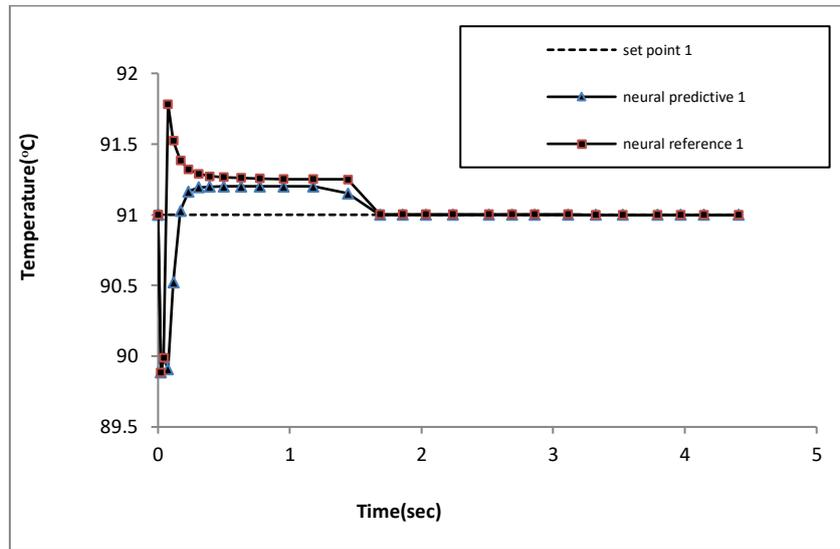
**Fig. 20** responses of the Temperature, which are related to 1st evaporator under the neural predictive and neural reference controllers to the step changes in the feed flow rate between 10,000 and 11,000kg/hr at 91°C set point.
