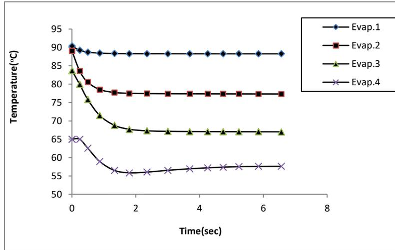
**Fig.14** evaporators of the temperature responses to the step-changes in the feed flow rate between 10,000 and 11,000kg/hr.
