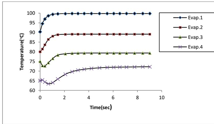
**Fig. 15** The temperature response evaporators to the step-changes in the feed of temperature between 75°C to 85°C.
