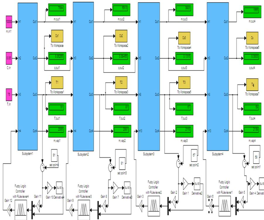
**Fig.9** Fuzzy logic control for each one of the evaporators in the caustic soda system.
