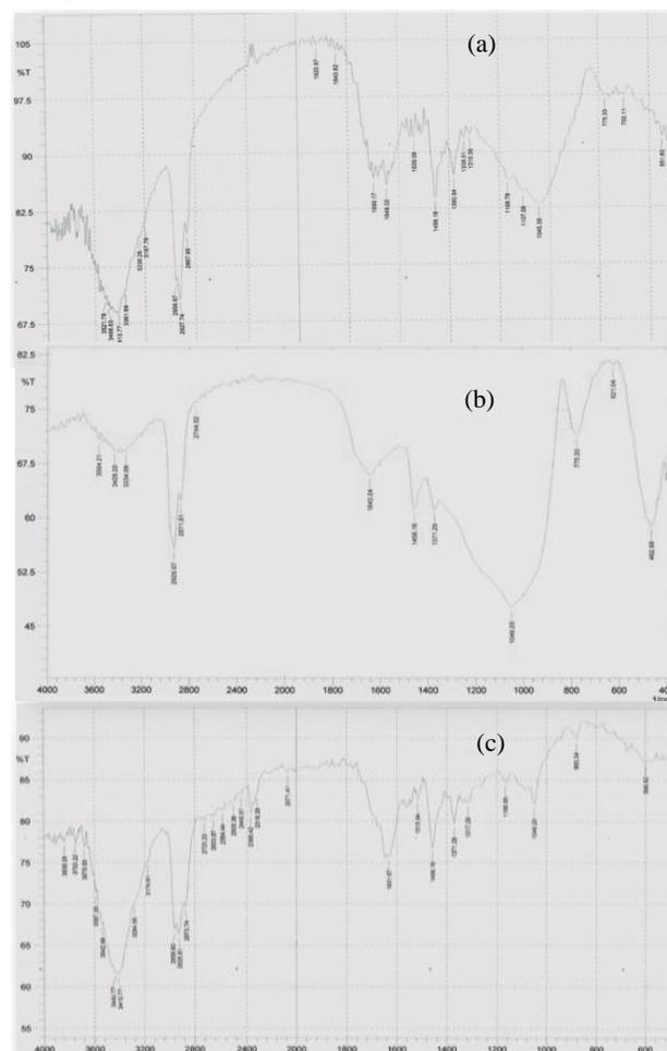
**Figure (3): FTIR spectra of (a) pure polyaniline, (b) PANI/TiO<sub>2</sub>nanocomposite with 1wt% TiO<sub>2</sub>, (c) PANI/TiO<sub>2</sub>nanocomposite with 5wt% TiO<sub>2</sub>.**
