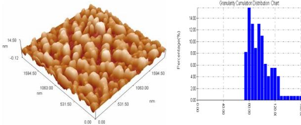
**Figure (6): AFM photographs of 5wt% of  $\text{TiO}_2$  in PANI/ $\text{TiO}_2$  thin film surface, 3D image and size distribution of  $\text{TiO}_2$ /PANI.**
