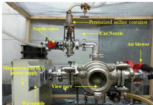
**Figure(2):Photograph of microwave plasma system for PANI/ $TiO_2$  nanocomposite thin films deposition.**
