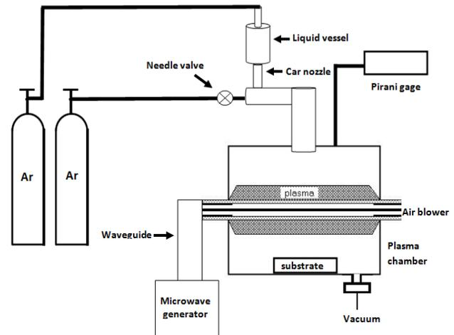
**Figure (1):Schematic diagram of the experimental arrangement.**
