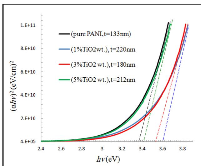
**Figure (4):** Variation of  $(\alpha hv)^2$  with photon energy  $(hv)$  of pure PANI and PANI/TiO<sub>2</sub> nanocomposite thin films of different concentrations of TiO<sub>2</sub>.
