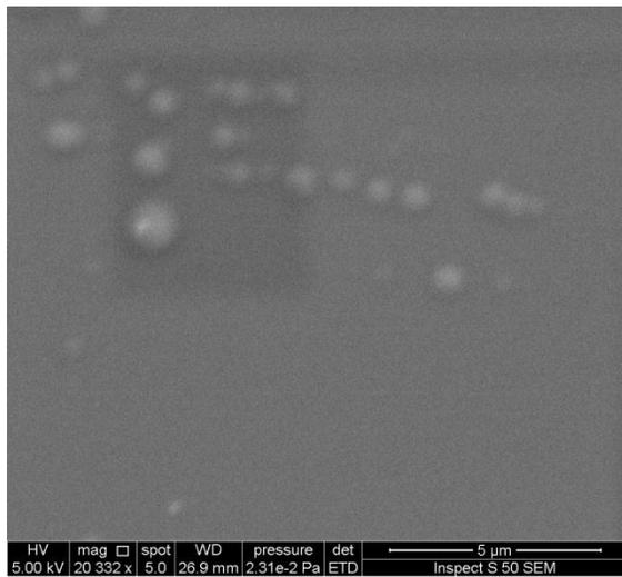
**Figure (7): SEM image of 1wt%  $\text{TiO}_2$  in PANI thin film.**
