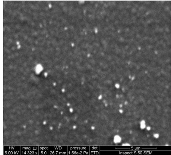
**Figure (8): SEM image of 5wt%  $\text{TiO}_2$  in PANI thin films.**
