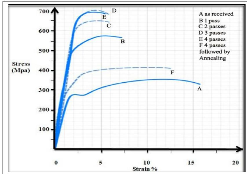
**Fig. 5. Stress-strain curve of unprocessed and ECAPed brass alloy samples.**
