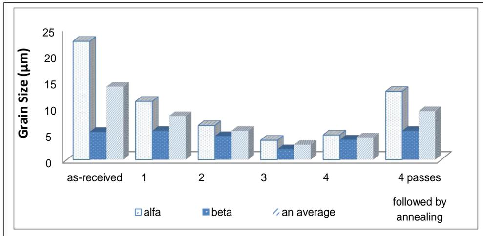
Fig. 3. Grain size distribution of brass alloy deformed by ECAP in different conditions.
