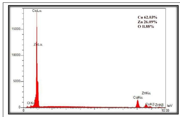
Fig. 1. EDS analysis of Cu-30Zn alloy used in this study.
