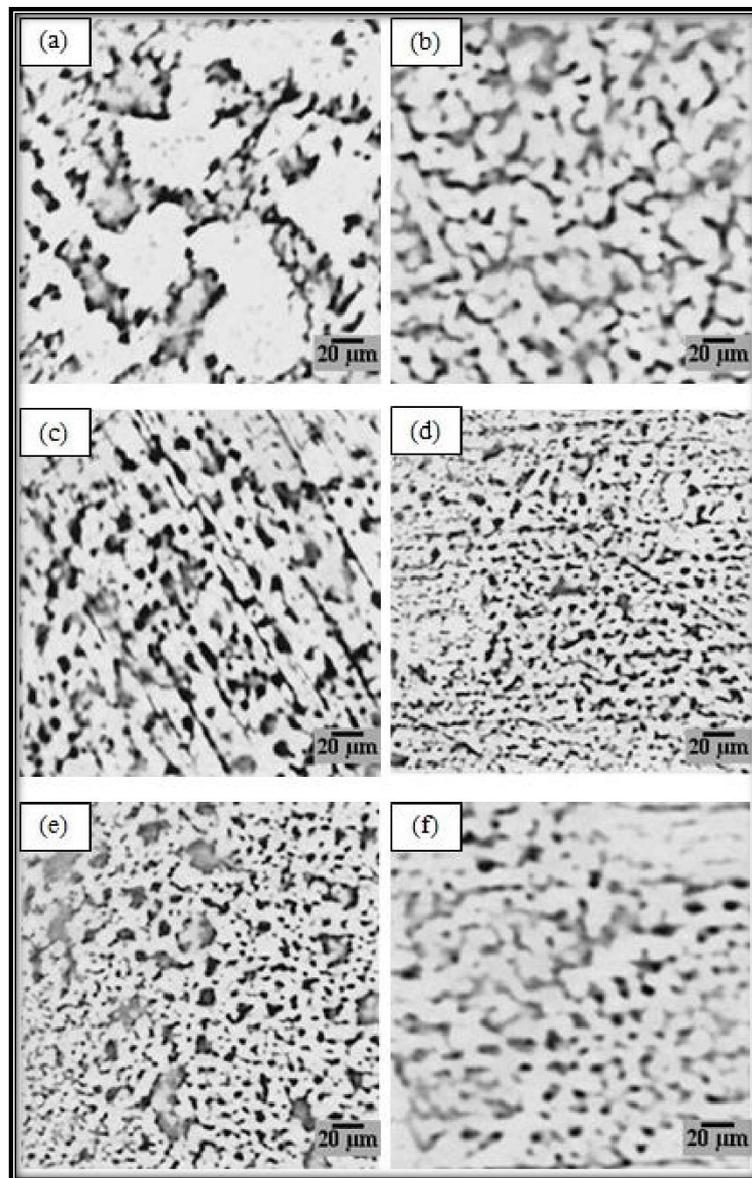
**Fig. 2.** Optical microstructures (1000 X) of brass alloy samples: (a) as-received, (b) 1 pass, (c) 2 passes, (d) 3 passes, (e) 4 passes and (f) 4 passes followed by annealing.
