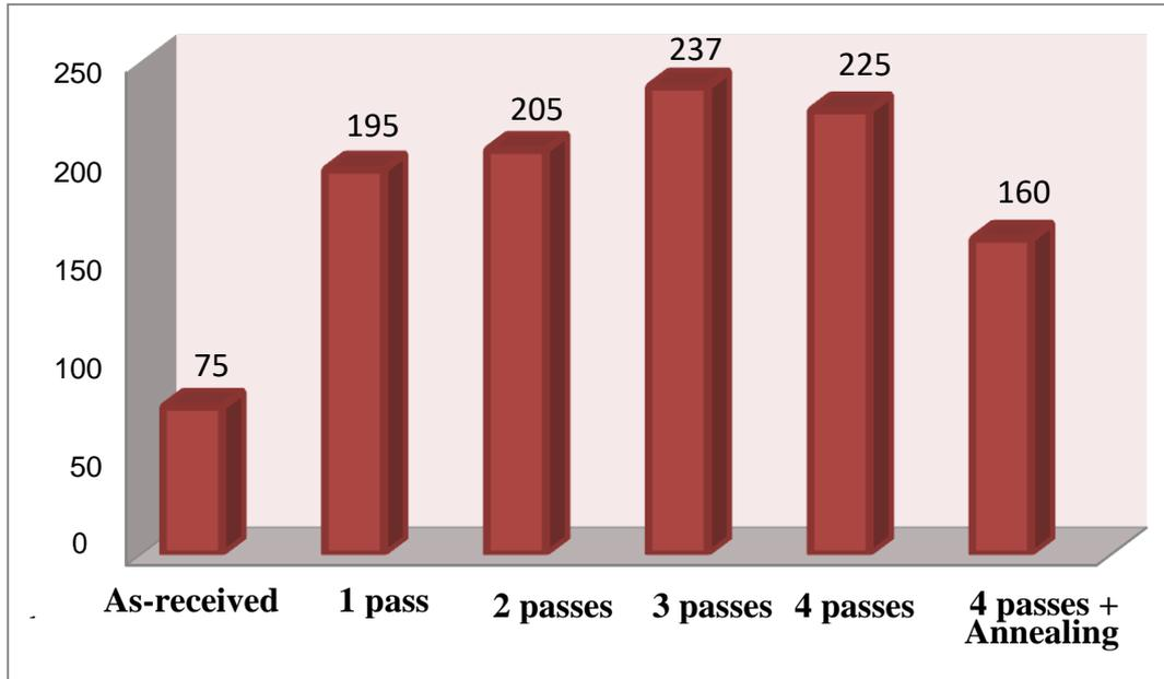
**Fig. 4. Variations of micro-hardness for brass alloy deformed by ECAP in different conditions.**
