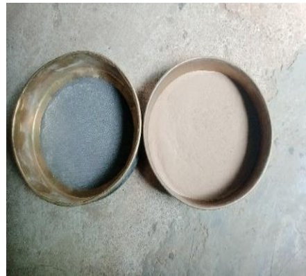
Fig. 1b. Ground melon seed husk and mesh sieve.
