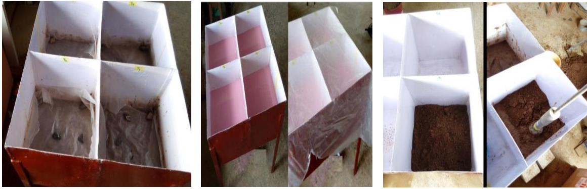
Fig. 5. Placing and compaction procedures.
