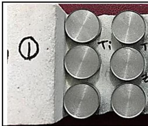
Fig. 1. Pure Ti and Ti-15Zr alloy samples produced by PM technique.
