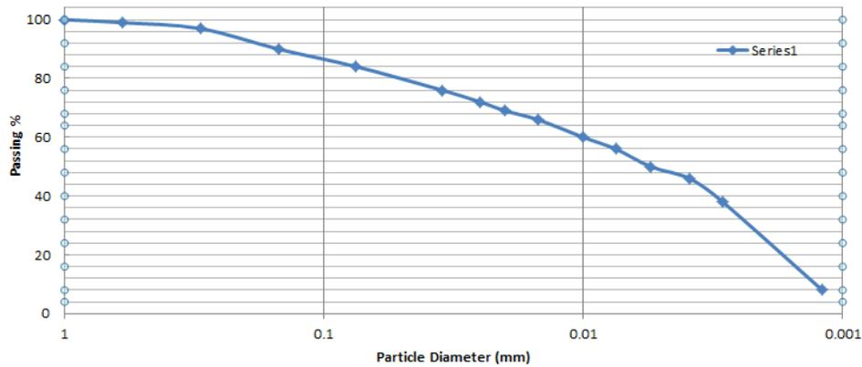
Figure (1). Grain Size of Soil Used
