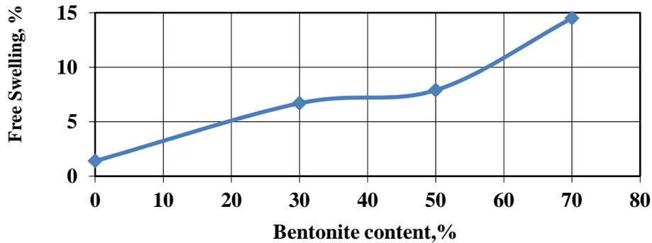
Figure (7). Free swelling versus Bentonite content for all types of soil used
