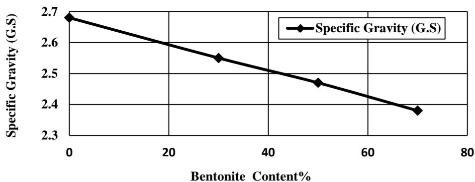
Figure (2). Effect of Bentonite content on specific gravity for soil used
