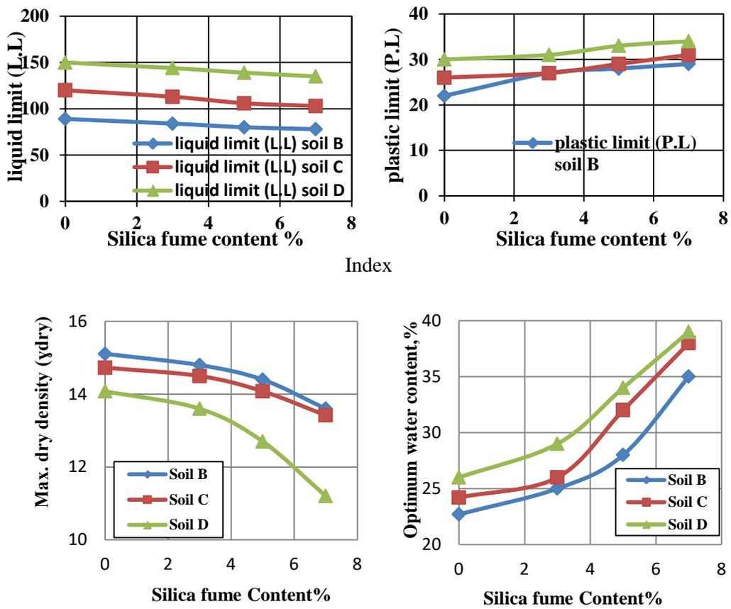
Figure (11). Effect of silica fume content on Compaction parameters
