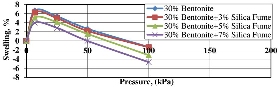
Figure(12). Swelling percent versus pressure for soil B
