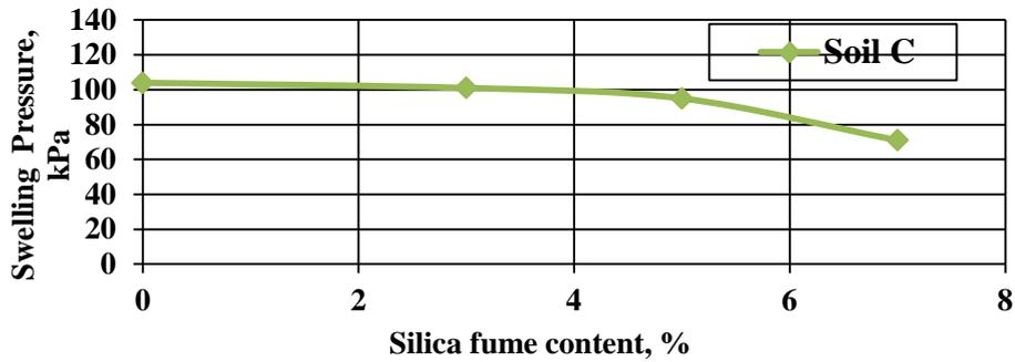
Figure(16). Swelling pressure versus silica fume content for soil C
