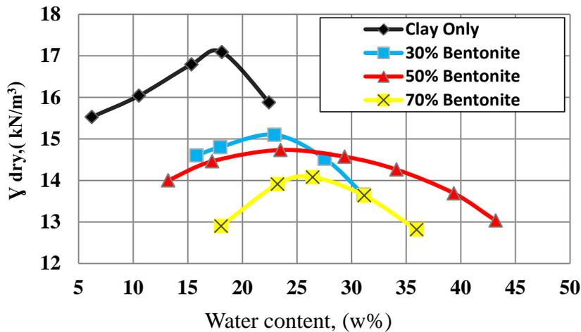
Figure (4). Relationship between water content versus dry density
