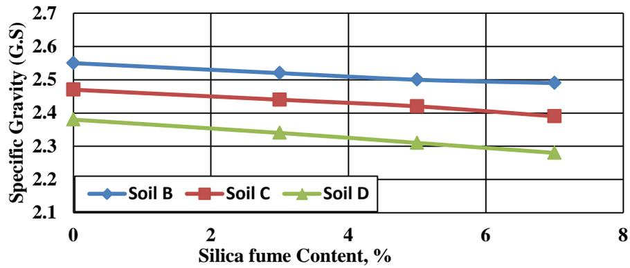
Figure (9). Effect of silica fume content on specific gravity
