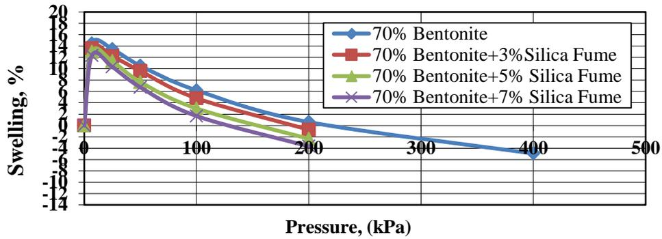
Figure(18). Swelling percent versus pressure for soil D
