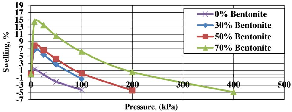
Figure (5). Swelling percent versus pressure for all types of soil used
