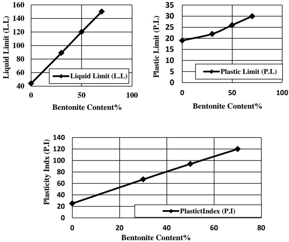
Figure(3). Effect of Bentonite content on L.L,P.L &P.I
