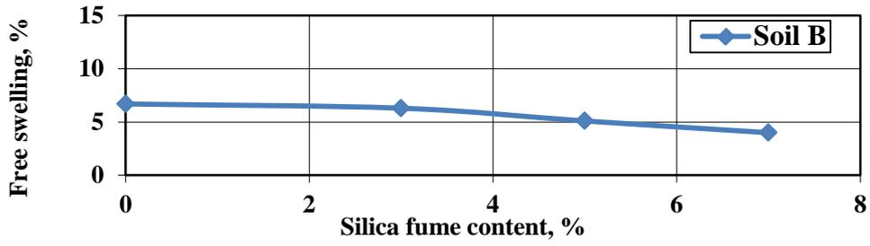
Figure(14). Free swelling versus silica fume content for soil B
