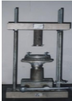
**Plate(1). Unconfined compression apparatus used for static compaction**
