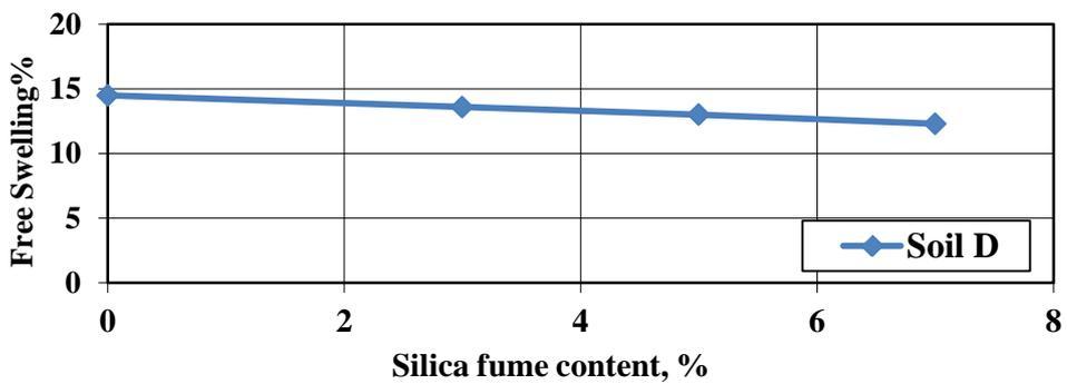
Figure(20). Free swelling versus silica fume content for soil D
