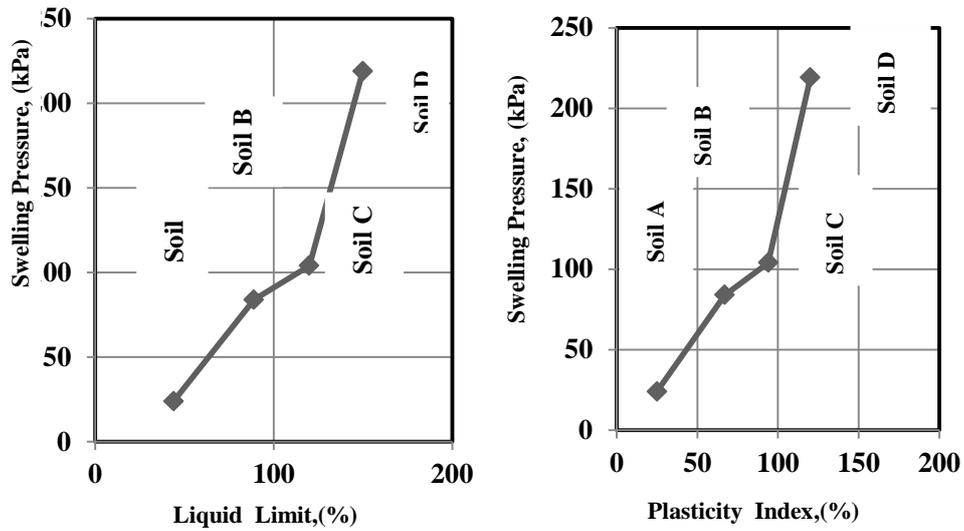
Figure (8). Effect of Liquid limit & Plasticity Index on Swelling Pressure
