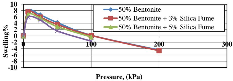
Figure(15). Swelling percent versus pressure for soil C
