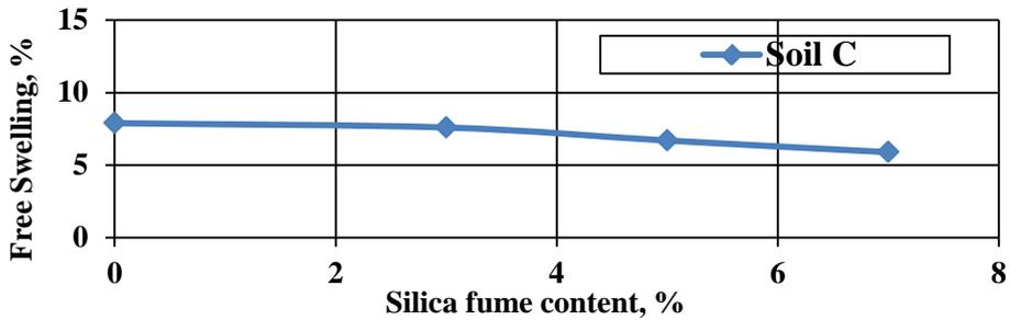
Figure(17). Free swelling versus silica fume content for soil C
