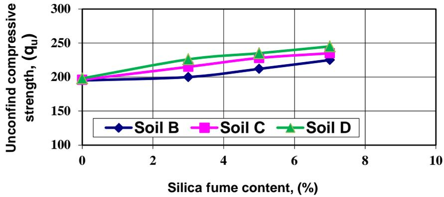
Figure (12). Effect of silica fume content on Compressive strength
