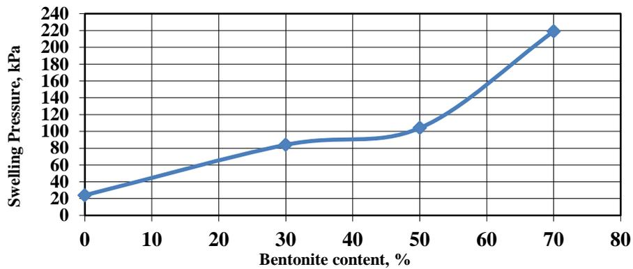
Figure (6). Swelling pressure versus Bentonite content for all types of soil
