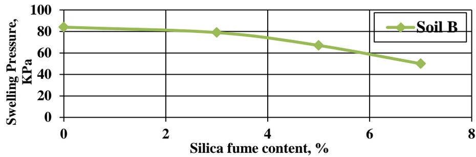
Figure(13). Swelling pressure versus silica fume content for soil B
