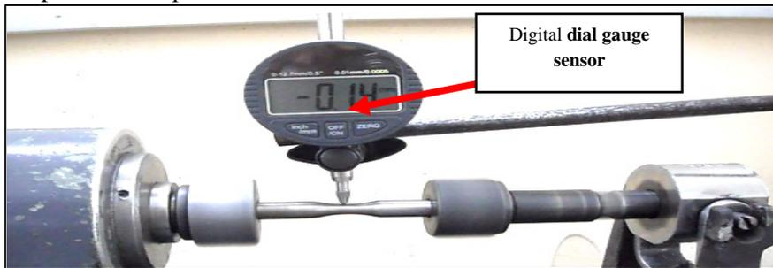
**Figure (4) the sensor holding on the test rig**
