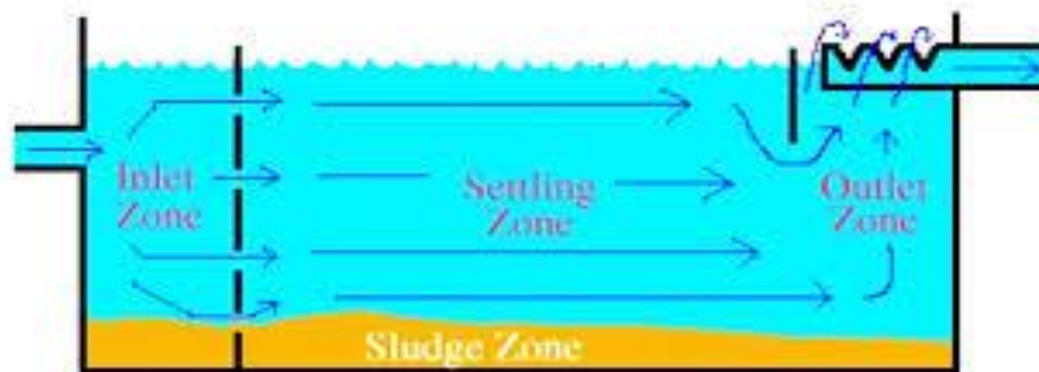
Fig(2):Primary settling basin
