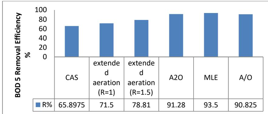
**Figure (2) BOD<sub>5</sub> removal efficiency for different systems**
