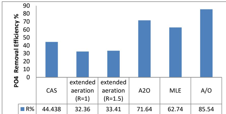
**Figure (7) PO<sub>4</sub> removal efficiency for systems**
