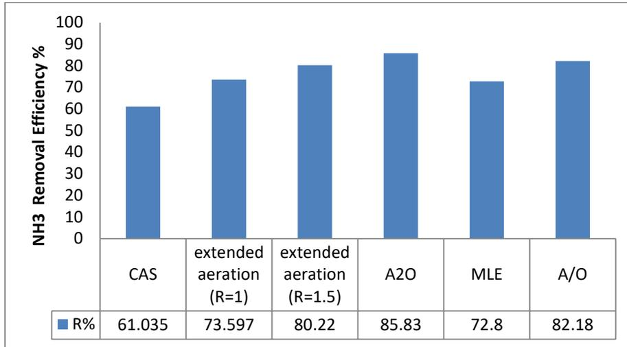
**Figure (4) :NH<sub>3</sub> removal efficiency for different systems**
