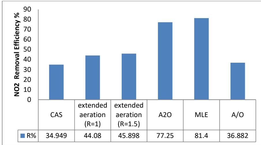
**Figure (6) NO<sub>2</sub> removal efficiency for different systems**
