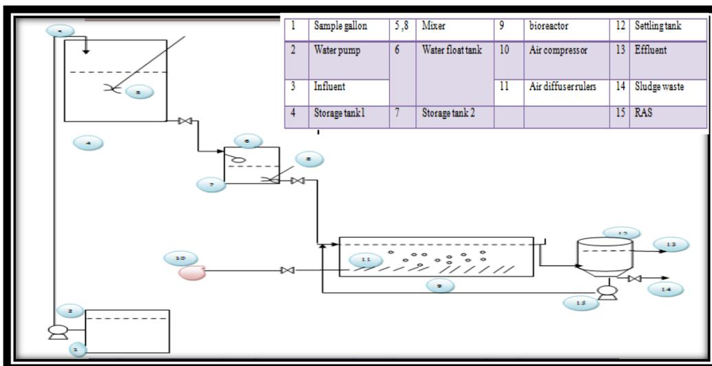
**Figure (1) A schematic diagram of the biological system**
