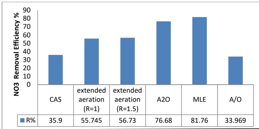
**Figure (5) NO<sub>3</sub> removal efficiency for different systems**
