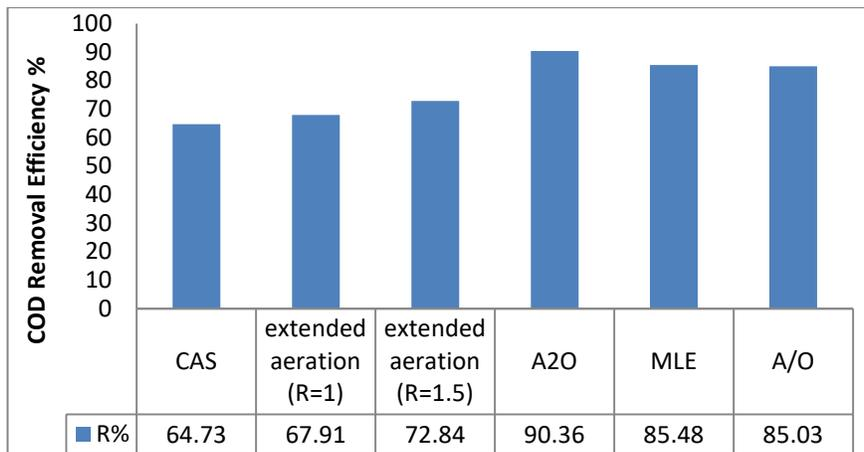
**Figure (3): COD removal efficiency for different systems**
