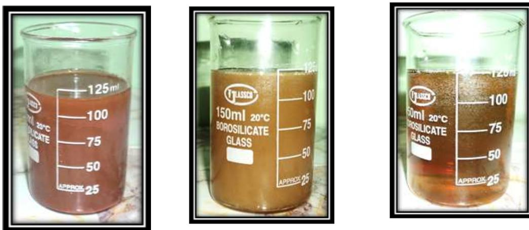
Fig.1 Show nanofluids for Cu+Oil, ZrO<sub>2</sub>+Oil and Oil
