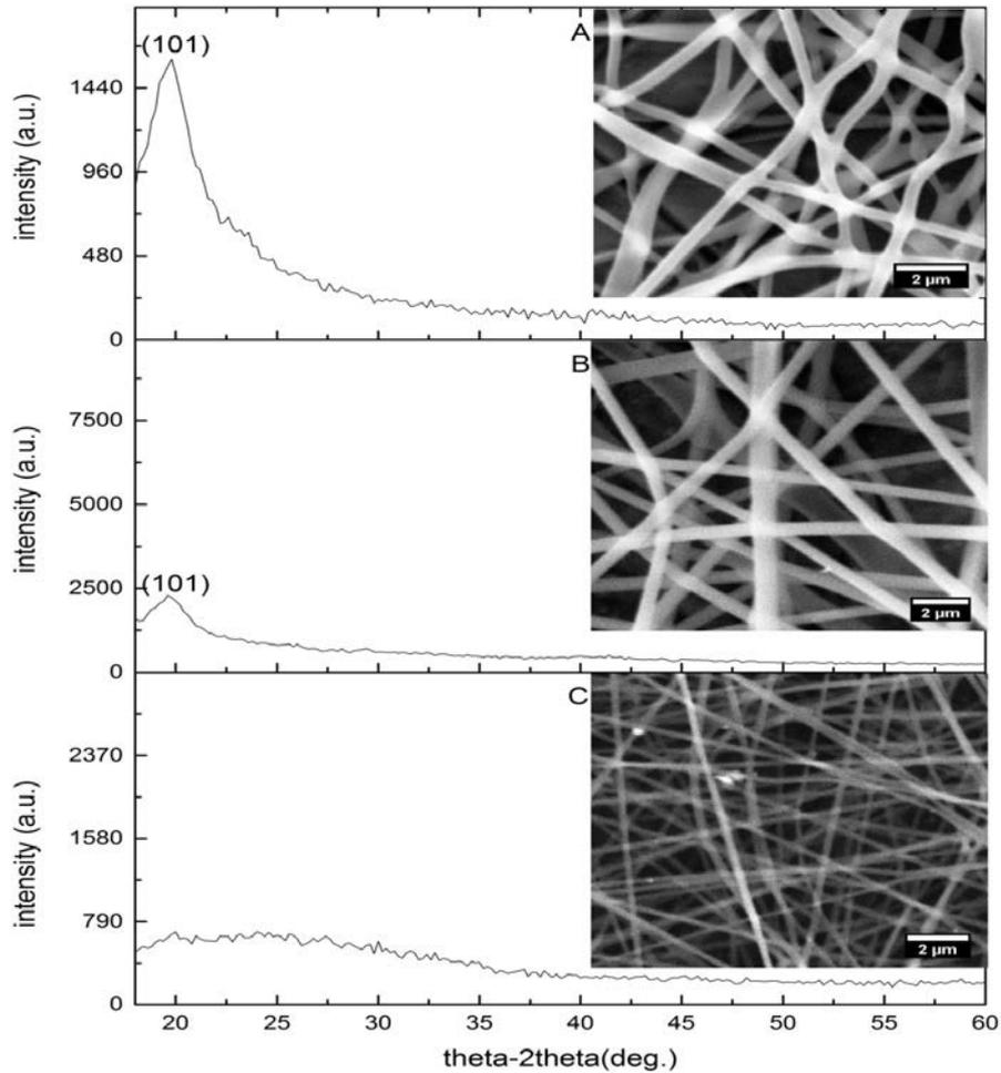
**Figure (2) XRD curve for fibers samples with different mass ratio. .a) PVA pure
