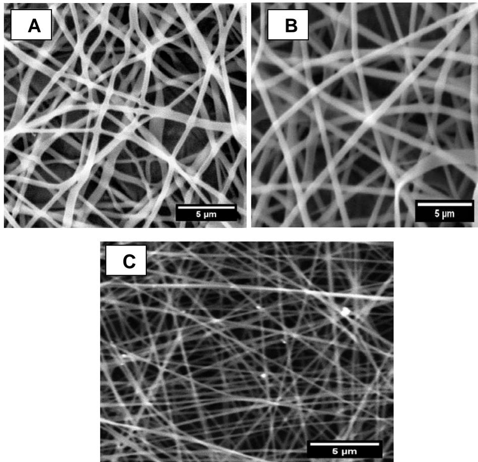
**Figure (3) SEM images of (a) electrospun PVA nano-fibers membrane, (b) electrospun PVA-1%TiO<sub>2</sub> membrane, (c) electrospun PVA- 3%TiO<sub>2</sub> membrane,**
