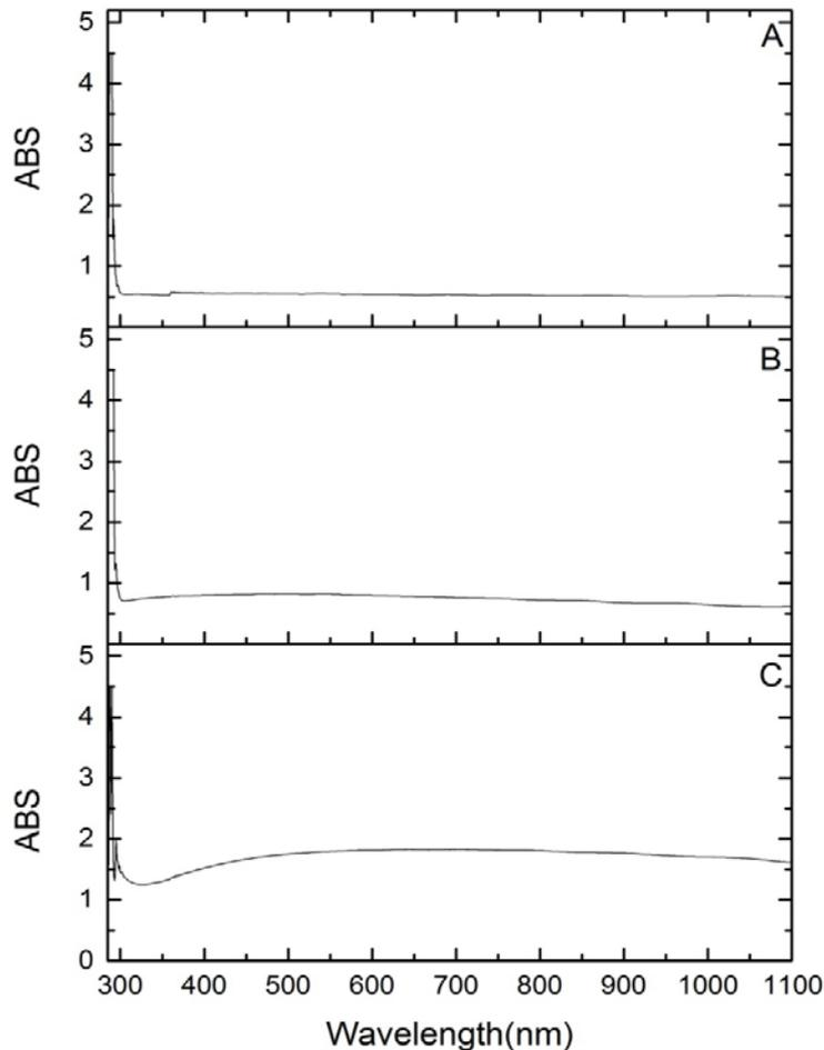
**(4) Figure show absorption properties of polymeric membranes pure and doped with different concentrations of TiO<sub>2</sub>.**
