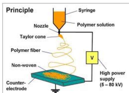
**Figure (1) Electrospinning setup and its product: non-woven fiber mat.**
