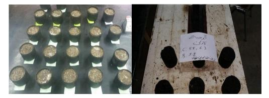
Figure 2. Part of the prepared cylindrical specimen for indirect tensile strength ratio test and index of retained strength.
