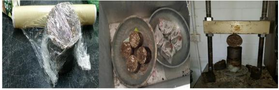
**Figure 3.** Wrapping the specimen with a plastic sheet, storage in freezer and the test apparatus (indirect tensile strength ratio test).
