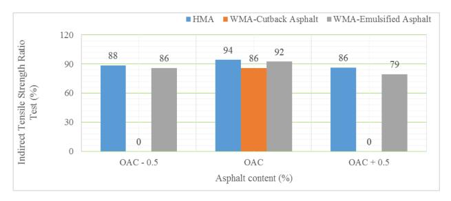
**Figure 6.** Effect of asphalt type and content on indirect tensile strength ratio.
