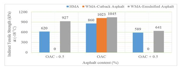
**Figure 5.** Effect of asphalt content on the indirect tensile strength under moisture damage.
