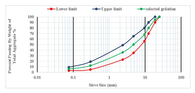
Figure 1. Gradation of the aggregates for binder course layer according to SCRB, 2003.
