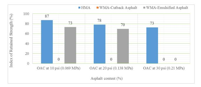
**Figure 7.** Effect of mixture types on the index of retained strength at different levels of stress.
