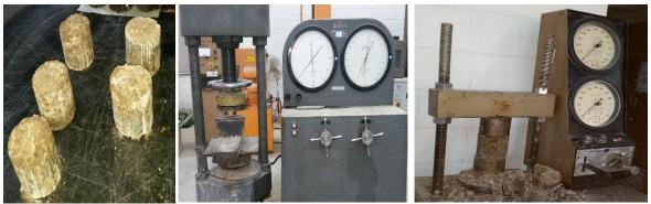
Figure 4. Part of the prepared specimens and the test apparatus (index of retained strength).
