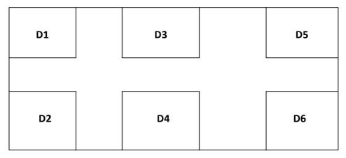
The above layout conforms to the rectangular floor plan of the plant and also places the assigned facilities adjacent to each other with an aisle of 2 meters width between them.
