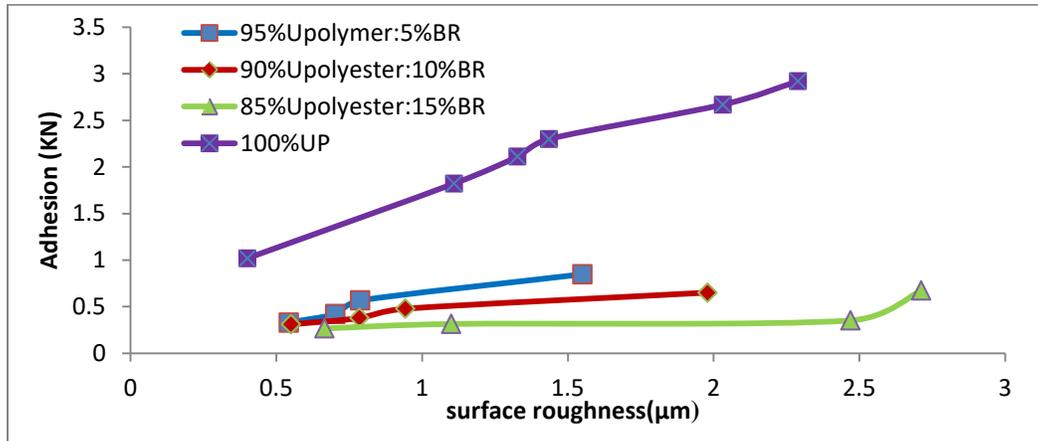
Figure (7) the effect of surface roughness of sherardizing coating on adhesion force for (UP: BR) blend and sherardizing coating low carbon steel.
