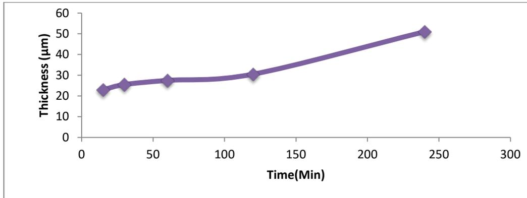
**Figure (3) Sherardizing thickness as a function of treatment time.**
