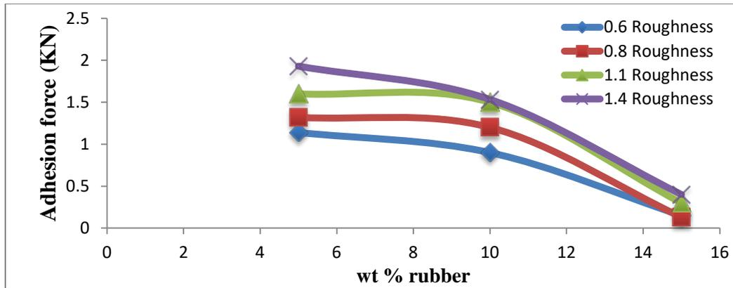
**Figure (8) The effect of rubber content on adhesion force for different values of surface roughness (UP : NBR ).**
