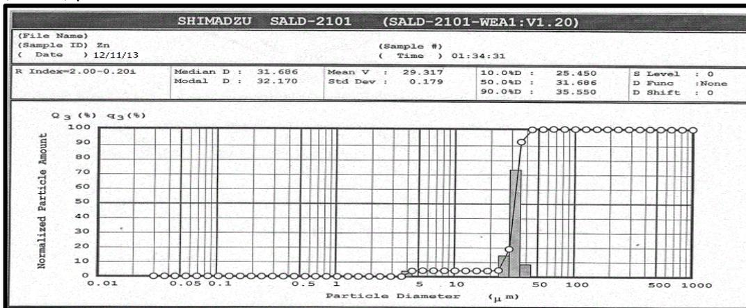
**Figure (1) Particles size distribution of zinc powder**
