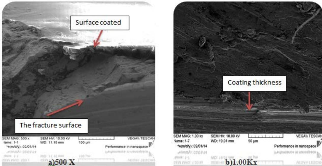
**Figure (12): SEM of sherardizing coating at different magnifications.**
