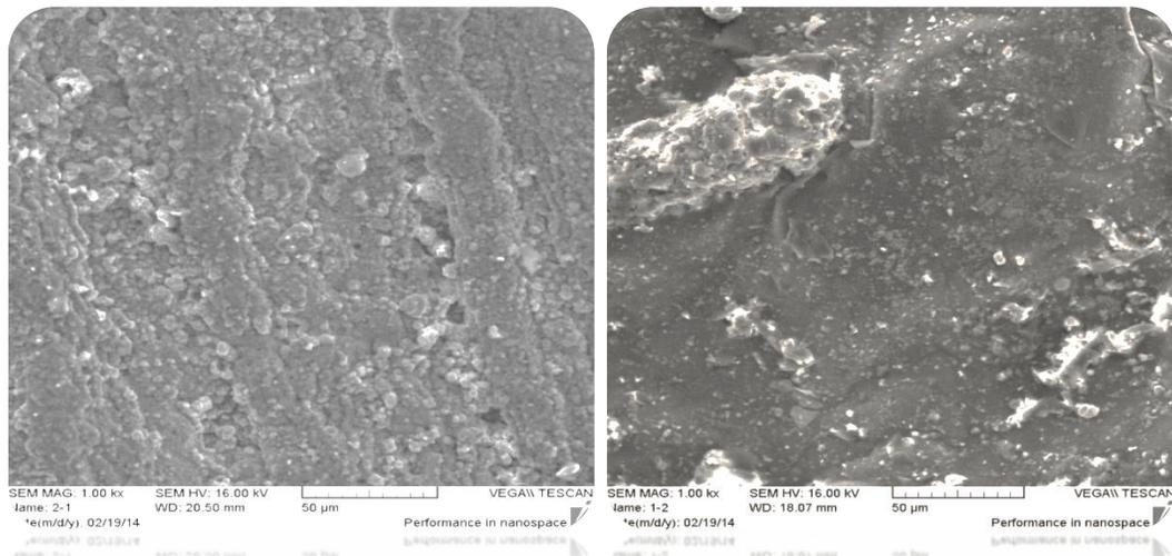
**Figure (13) surface morphology of coating samples by polymer blends (a) (90%UP: 10%BR) and (b) (90%UP:10%NBR) at 1000X magnifications.**
