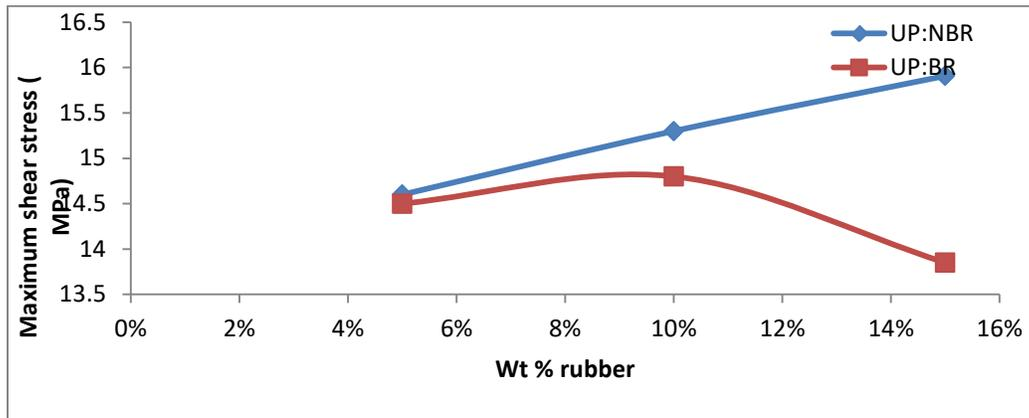
**Figure (11)** The maximum shear stress of sherardized low carbon steel as a function of BR or NBR content in the polymer blends coating layer.
