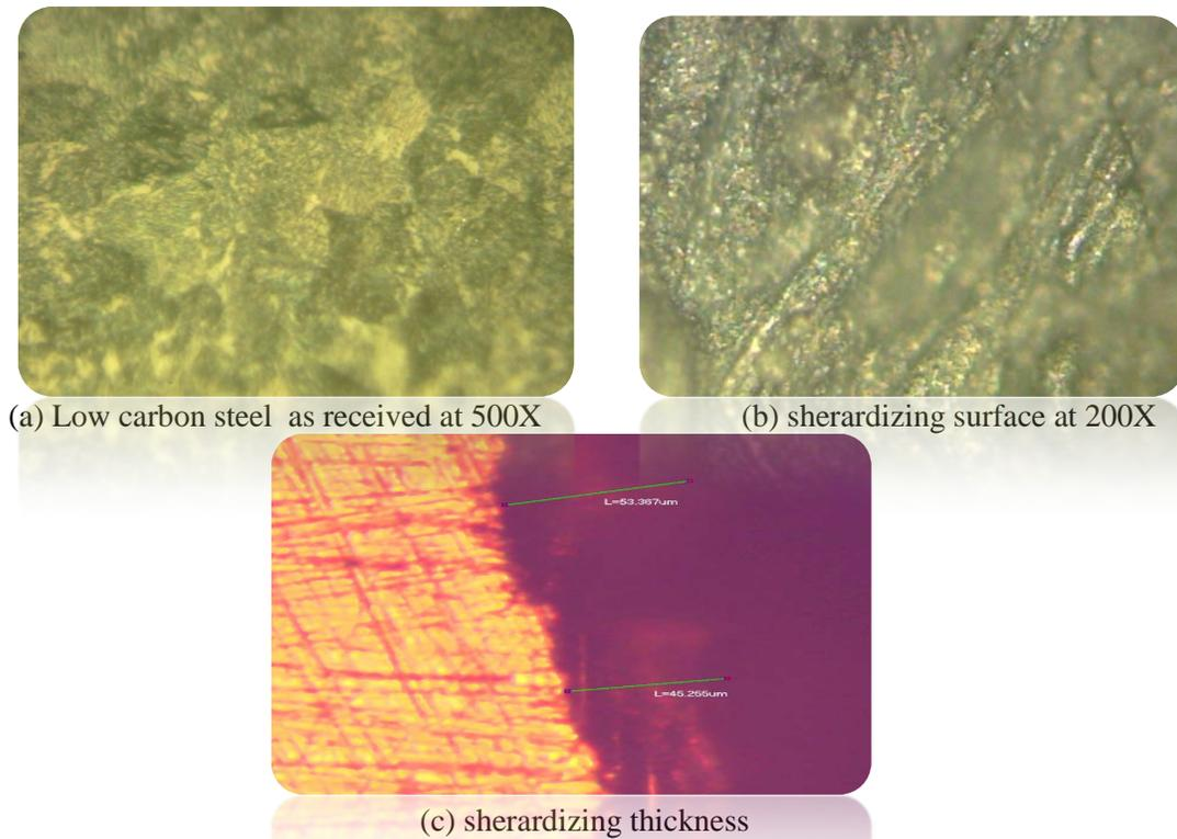
**Figure (2) Optical micrographs of as received (low carbon steel) sample and sherardizing coating. A: Low carbon steel as revised at 500X magnification, B: Sherardizing surface at 200X magnification, C: Sherardizing thickness.**
