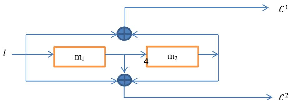
**Figure (2): Convolutional Encoder**
