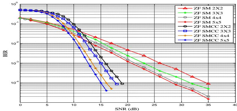
Figure (13): SM with CC of 2/3 code rate
