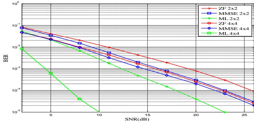
**Figure(4): SM of 4x4 and 2x2 with modulation order =2**
