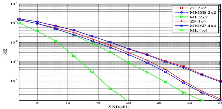
**Figure (5): SM of 4x4 and 2x2 with modulation order =4**
