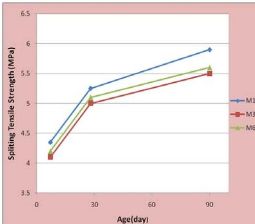
**Figure(4):** Development of splitting tensile strength with age for mixes contain crushed quartzite.
