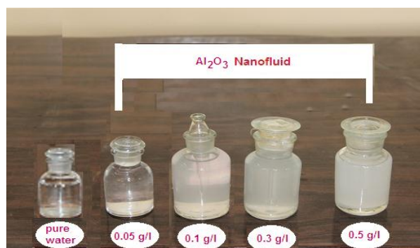
Figure (6) Photographs of the water-Al 2 O 3 nano fluid preparation
