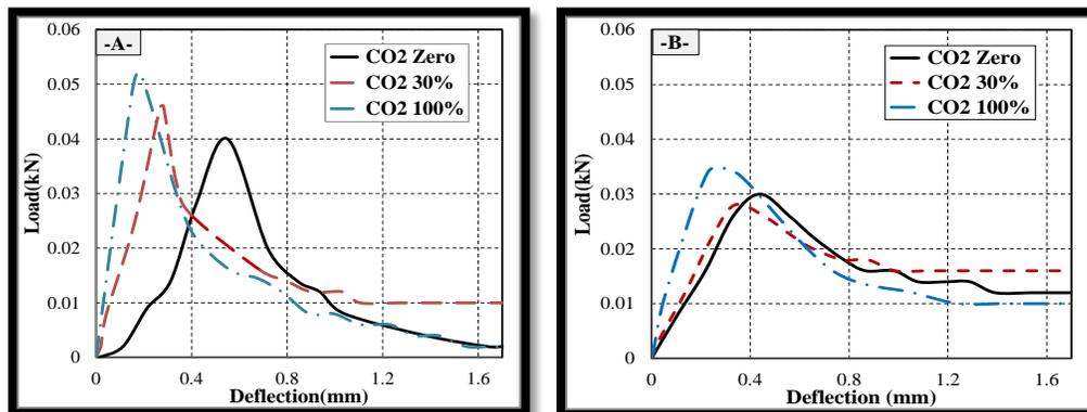
**Figure (5). Typical Load deflection curve characteristics of cement-bonded cellulose fiberboard; (A) Cellulose fiber/matrix=0.05, (B) Cellulose fiber/matrix=0.08.**
