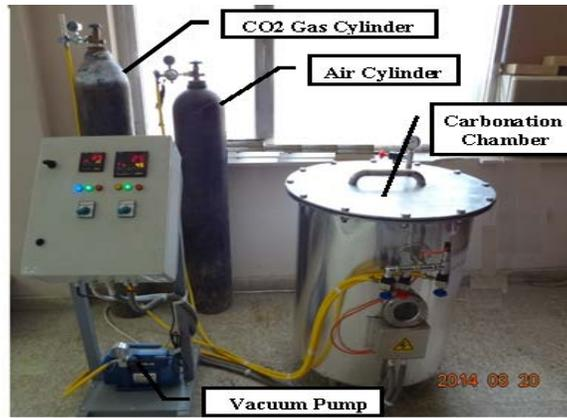
Figure(2). Processing system incorporating CO<sub>2</sub> curing.
