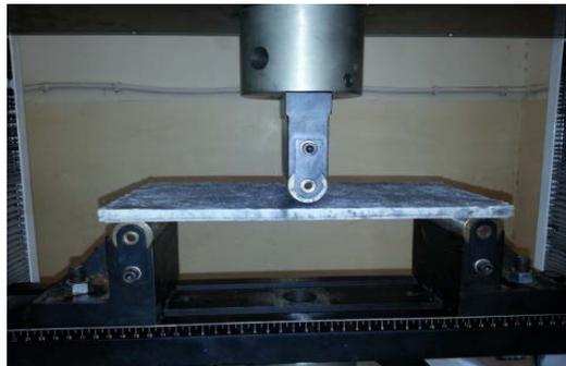
**Figure(4). Set-up of flexural test of the cement-bonded cellulose fiber-board (CBCB).**
