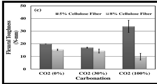
**Figure (7). Effects of various CO<sub>2</sub> concentrations on the flexural performance of cement-bonded cellulose fiberboard, (a) Flexural strength, (b) initial stiffness, and (c) flexural toughness.**
