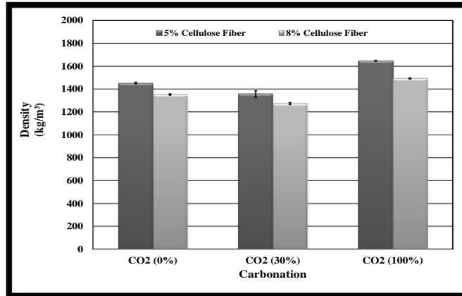
**Figure(8). Bulk density of cement-bonded cellulose fiber-board (CBCB) subjected to different CO<sub>2</sub>-curing concentrations.**
