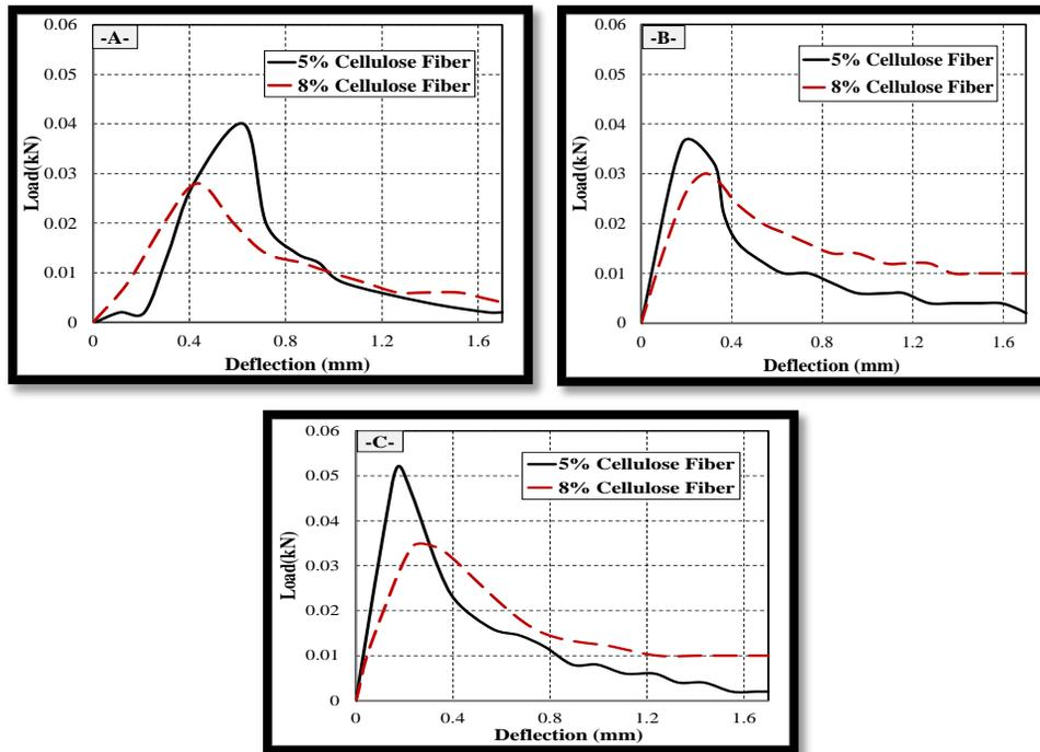
**Figure(6).Effects of various CO<sub>2</sub> concentrations on the L-D curve characteristics of cement-bonded cellulose fiberboard; (A) 0% CO<sub>2</sub> concentration, (B) 30% CO<sub>2</sub> concentration, (C) 100% CO<sub>2</sub> concentration.**
