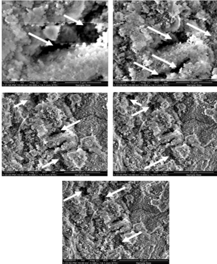
**Figure(10). SEM micrographs of the fractured surface of non-carbonated and 5% fiber/matrix ratio of fiber-cement composites, white arrows indicate porous areas.**
