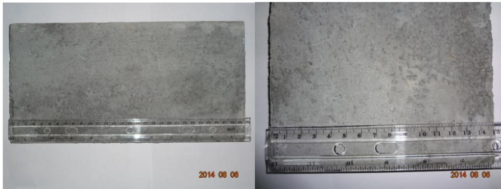
Figure(3). Typical appearance of cement-bonded cellulose fiberboard (CBCB).
