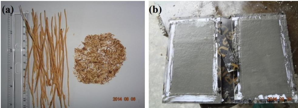
Figure(1). Appearance of cellulose date palm fibers (a) and produced boards (b).
