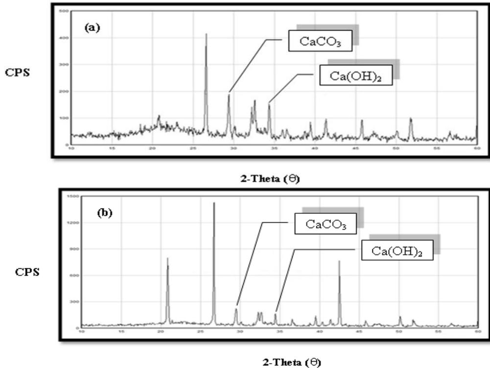
**Figure (9).** X-ray patterns after CO<sub>2</sub> curing 30% concentration for cement-bonded cellulose fiber-board; (a) cellulose fiber ratio 5%, and (b) cellulose fiber
