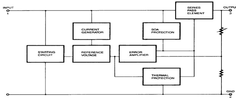
Figure (5): The Internal Block Diagram of the MC7812 [9].
