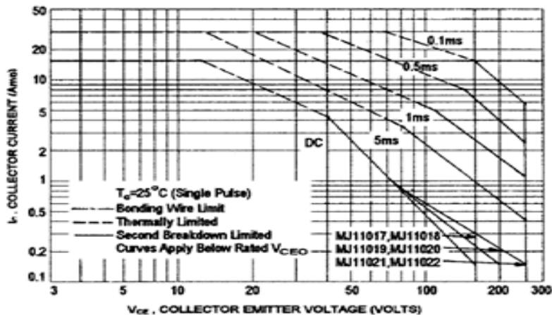
Figure (4): The Forward Bias Safe Operation Area of the MJ11021 Transistor.
