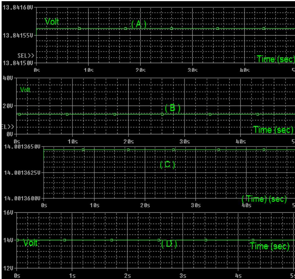
**Figure (8): The Output Voltage of the Charge Controller at Full-load for Four Input Voltages.**
