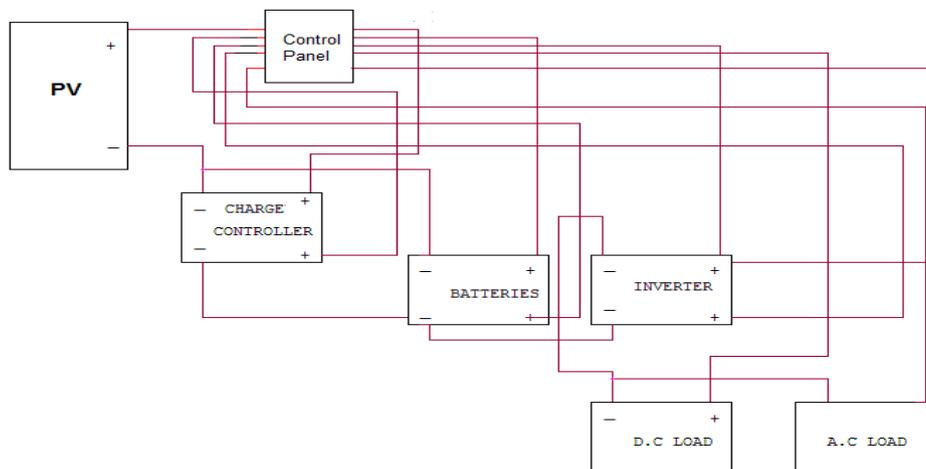
Figure (1): Block Diagram of a Typical Solar System.
