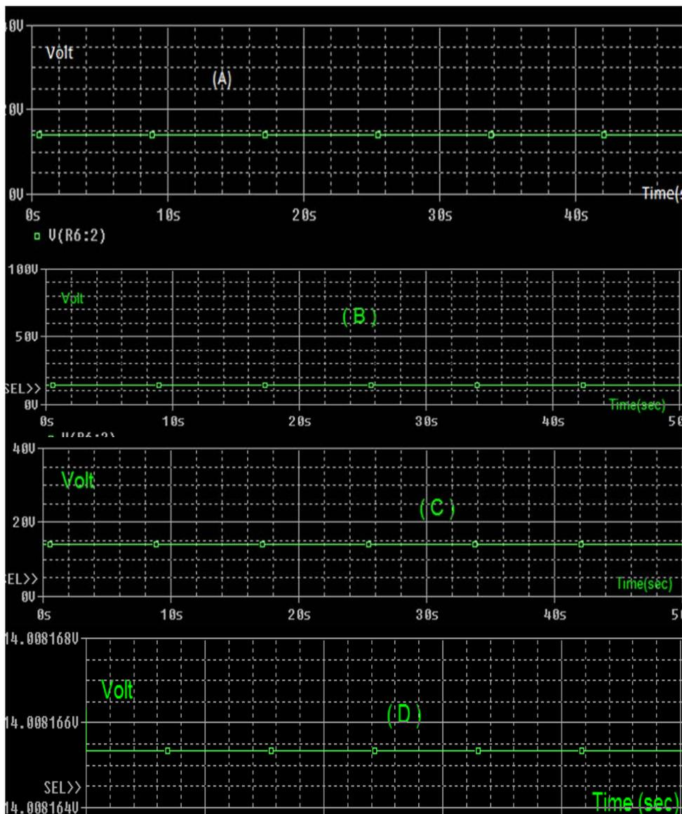
Figure (7): The Simulated Output Voltage of the Charge Controller with No-load at Four Input Voltages.
