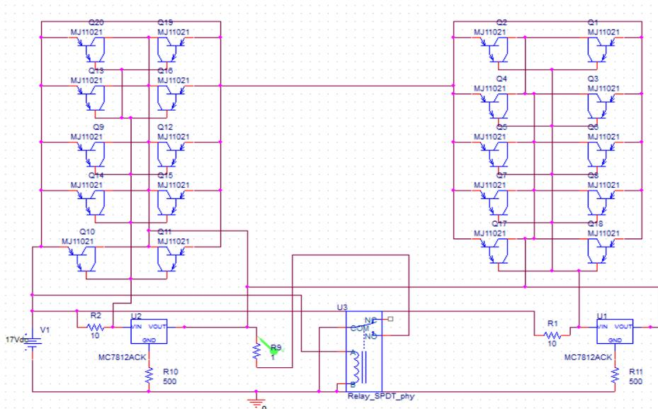
Figure (6): The Circuit Diagram of the Designed Charge Controller (14 V, 220 A).
