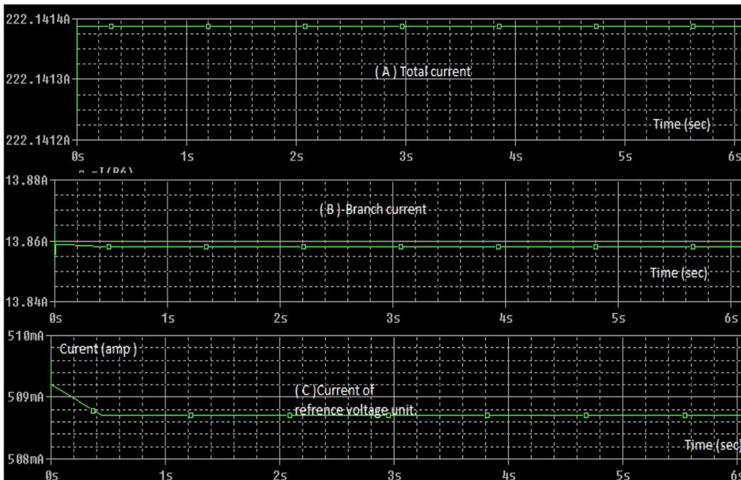
**Figure (9): Current traces of the charge controller.**
