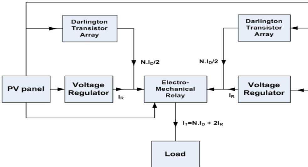
**Figure (2): Block Diagram of the Suggested Design of the Charge Controller.**
