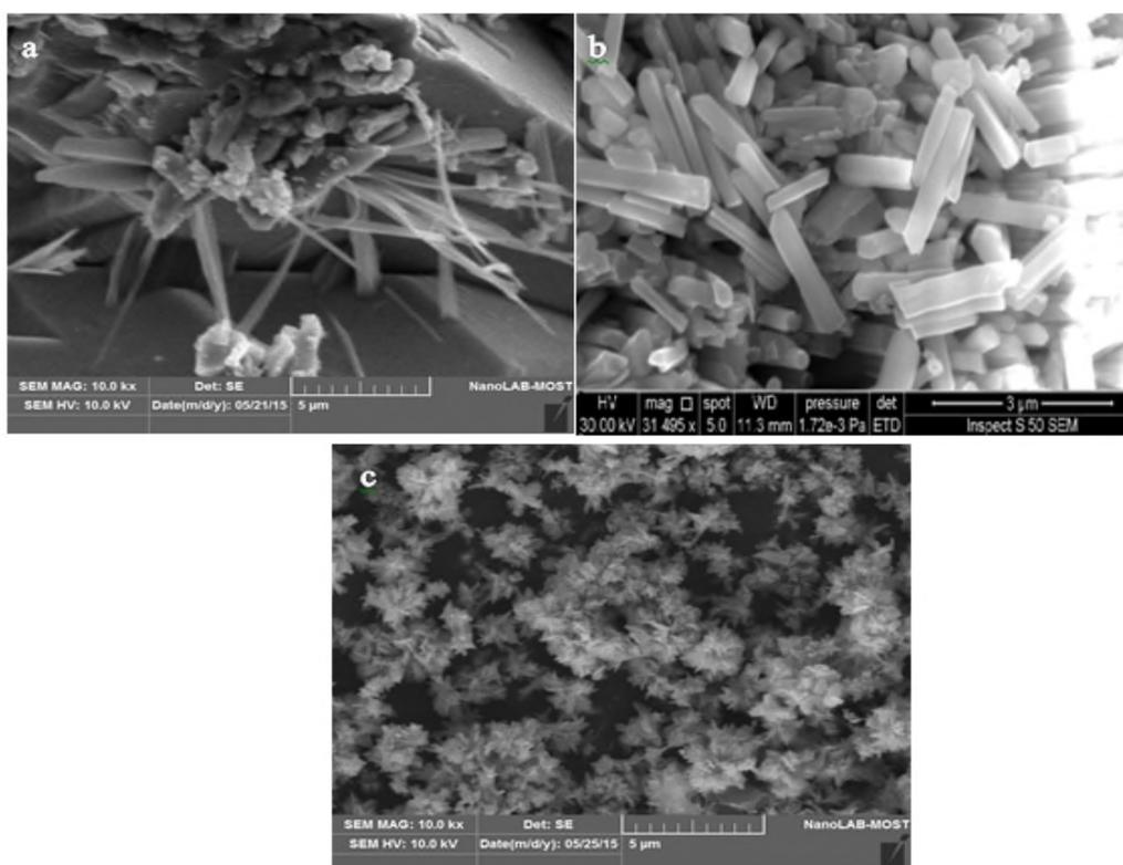
Figure( 3) The SEM images of the ZnO nano rods hydrothermally grown from one g of ZnO nanoparticles and (3M) NaOH aqueous at 90 °c for (a) 24 h, (b)48 h and (c) 72 h
