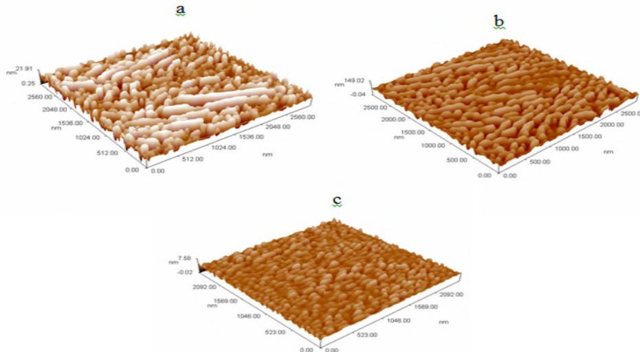
Figure( 2) AFM images of the ZnO nano rods hydrothermally grown from (1g) of ZnO nanoparticles and (3M) NaOH aqueous at 90 °c for (a) 24 h, (b)48 h and (c) 72 h
