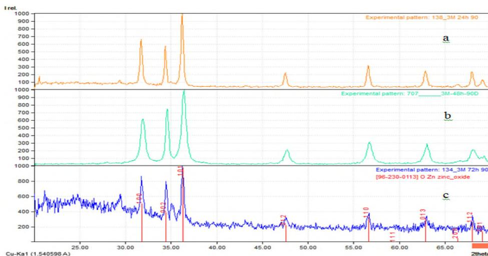
Figure (1 )XRD pattern of ZnO nano rods: (a) arrays as-prepared at 90 °C for 24 (b) as-prepared at 90 °C for 48 h; (c) as-prepared at 90 °C for 72 h
