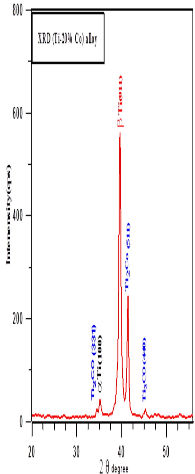
Fig.1: XRD patterns Ti-20%Co alloy uncoated.
