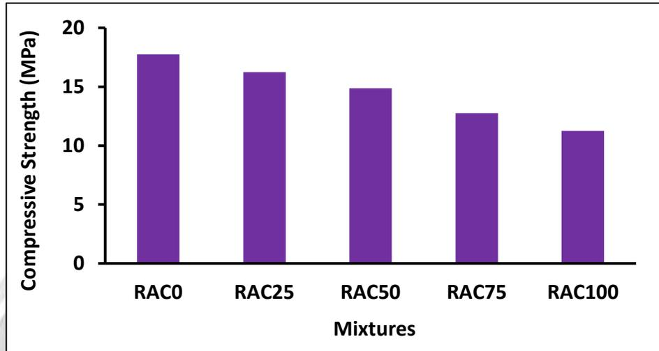
**Figure 5:** Compressive Strength of Various RAC Mixtures at 90 Days Immersed in 5%  $H_2SO_4$  Acid
