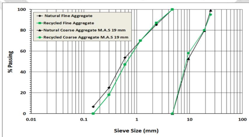
**Figure 1: Gradation of Natural Aggregates and Recycled Aggregates.**
