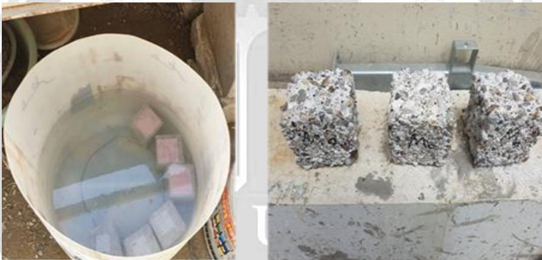
**Figure 2: Chemical Attack Resistance Test, A) Specimens under Full Immersion, B) Specimens after 90 Days of Immersion.**
