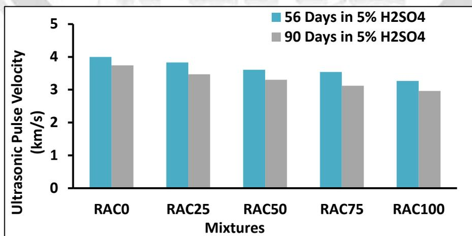
Figure 4: Ultrasonic Pulse Velocity of Various RAC Mixtures at 56 and 90 Days Immersed in 5%  $\text{H}_2\text{SO}_4$  Acid
