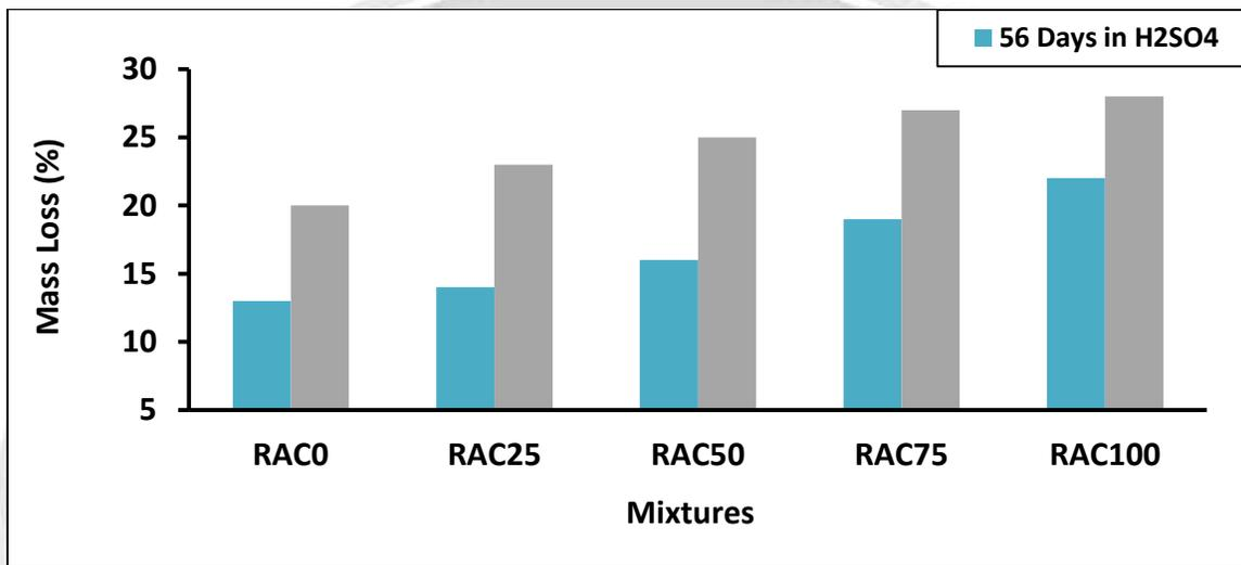
**Figure 3: Mass Loss of Various RAC Mixtures at 56 and 90 Days Immersed in 5%  $H_2SO_4$  Acid**
