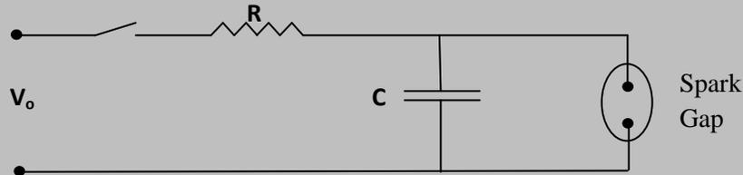
**Figure(1) A schematic representation of a capacitor charge-discharge circuit. The capacitor is discharged through a spark gap.**
