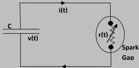
**Figure (2) A schematic representation of a capacitor discharge through a time variable resistance of a spark gap.**
