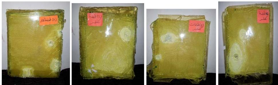
Figure (17): shows the geometry of front face deformation after ballistic test .
