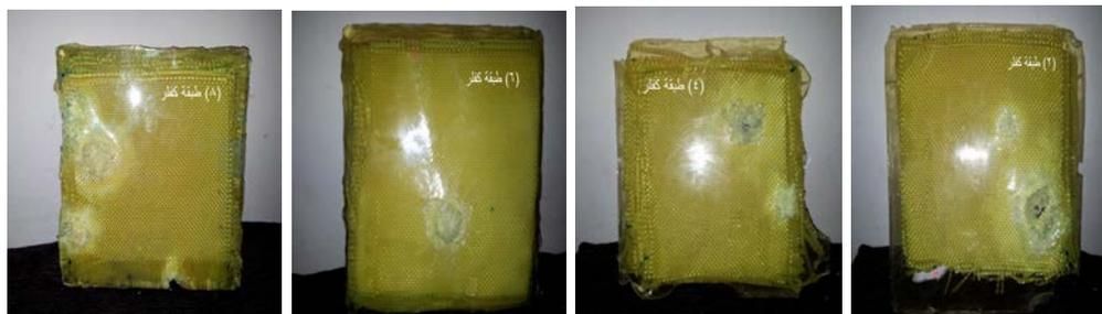
Figure (18): Shows the geometry of back face deformation after ballistic test.
