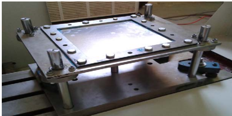
Figure. (2) Schematic representation of the experimental set up of TPIF process: the sheet metal blank, the blankholder, movable frame, post guide sliding bush and partial die
