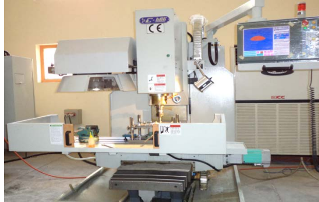
Figure. (1). 3-Axis CNC milling machine used in experimental work. (1) CNC milling machine. (2) Machine controller. (3) Tool holder. (4) Forming frame. (5) Forming tool.
