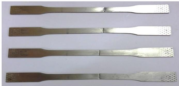
**Figure (2):** The specimens prepared for tensile tests
