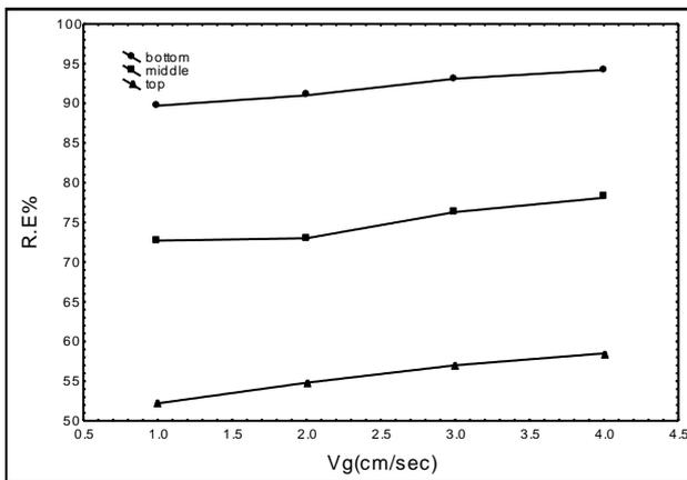
Figure (4) Effect of Gas Velocity on Removal Efficiency for Different Stage at Cf =15ppm of Caprylic acid
