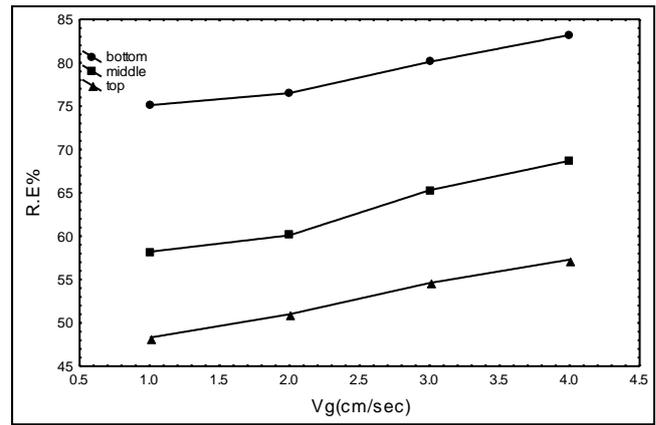
Figure (3) Effect of Gas Velocity on Removal Efficiency for Different Stage at Cf =10ppm of Caprylic acid
