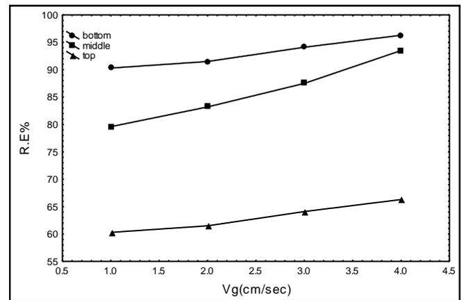
Figure (5) Effect of Gas Velocity on Removal Efficiency for Different Stage at Cf =20ppm of Caprylic acid
