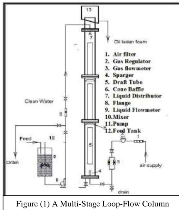
Figure (1) A Multi-Stage Loop-Flow Column
