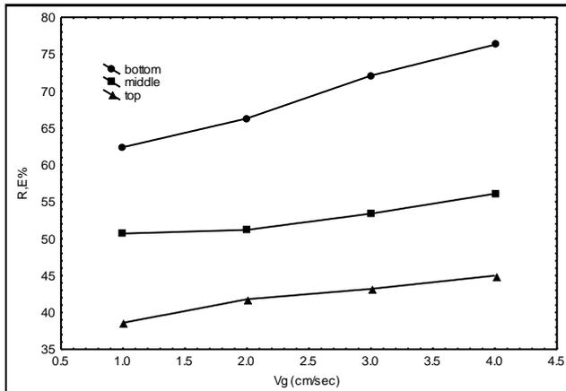
Figure (2) Effect of Gas Velocity on Removal Efficiency for Different Stage at Cf =5ppm of Caprylic acid
