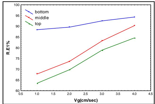
Figure (9) Effect of Gas Velocity on Removal Efficiency for Different Stage at Cf =20ppm of Hexanol
