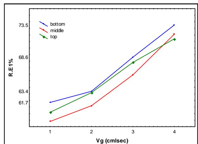
Figure (7) Effect of Gas Velocity on Removal Efficiency for Different Stage at Cf =10ppm of Hexanol
