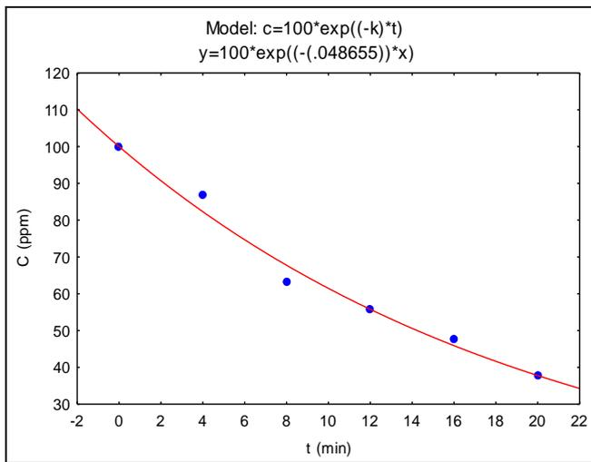
Figure (10) Example of (k) Estimation Using STATISTIC Software at Vg= 1cm/sec. and Cf=5 ppm of Caprylic Acid
