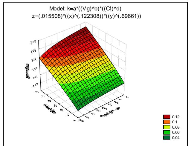
Figure (11) Relation of Kinetic Flotation Constant with Superfacial Gas Velocity and Frother concentration Using Caprylic Acid
