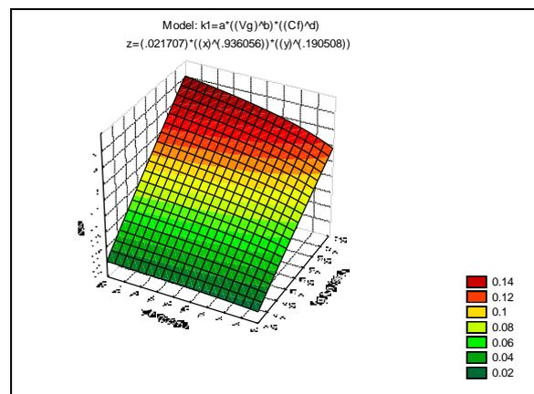
Figure (13) Relation of Kinetic Flotation Constant with Superfacial Gas Velocity and Frother concentration Using Hexanol
