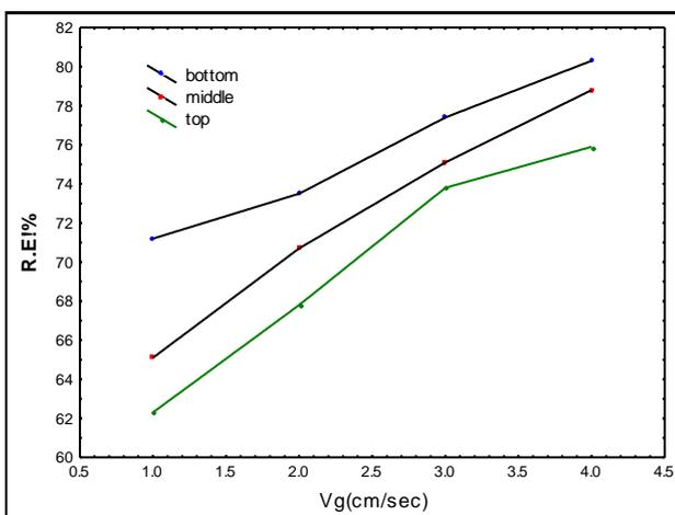
Figure (6) Effect of Gas Velocity on Removal Efficiency for Different Stage at Cf =5ppm of Hexanol
