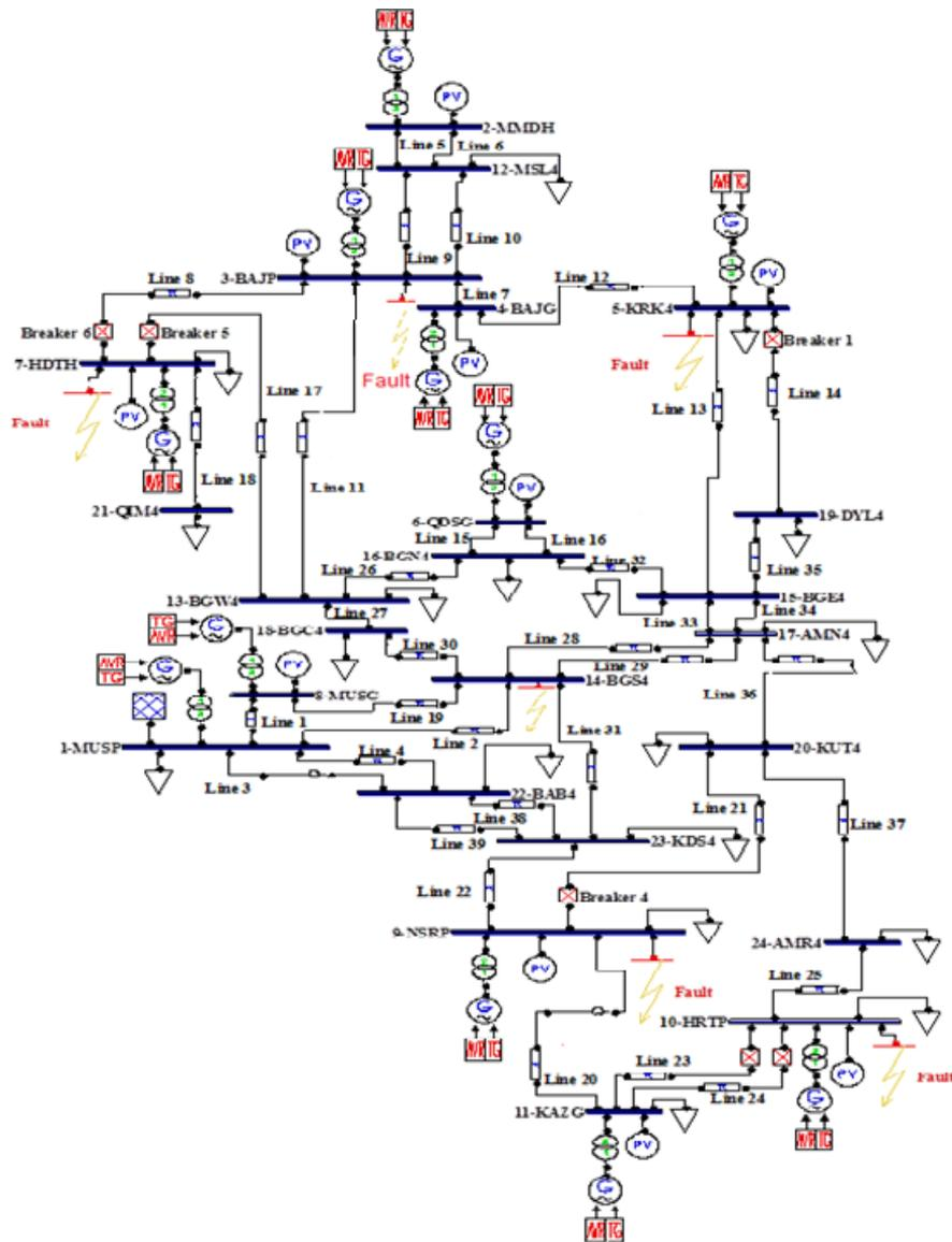
Figure (8) Iraqi (400kv) National Super Grid System(Insgs)
