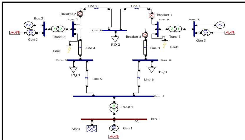
Figure (6) IEEE 3-machine, 9-bus system
