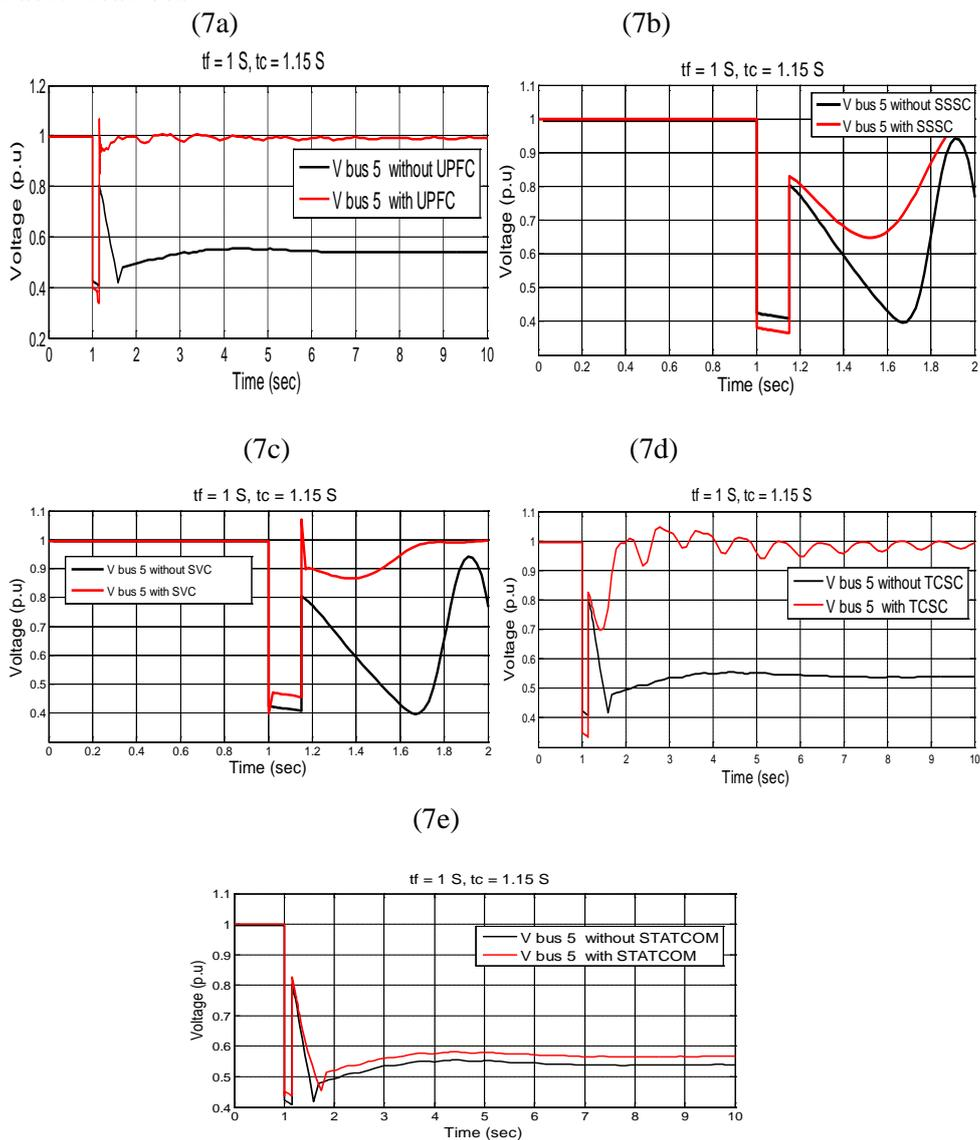
**Figure (7a,b,c,d,e) Voltage with and without UPFC,SSSC,STATCOM ,SVC,TCSC**
