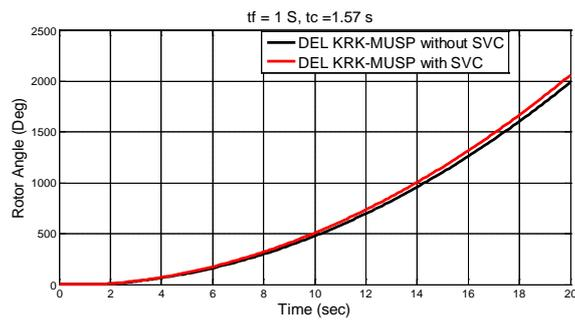
**Figure (10 a,b,c,d,e) Rotor angle difference of KRK with and without UPFC,SSSC,TCSC,STATCOM, SVC respectively.**
