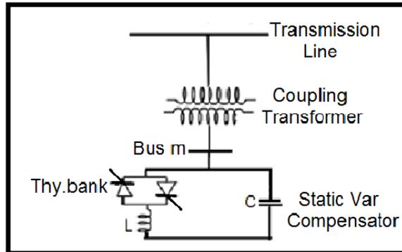
**Figure (1) SVC connected to a transmission line**
