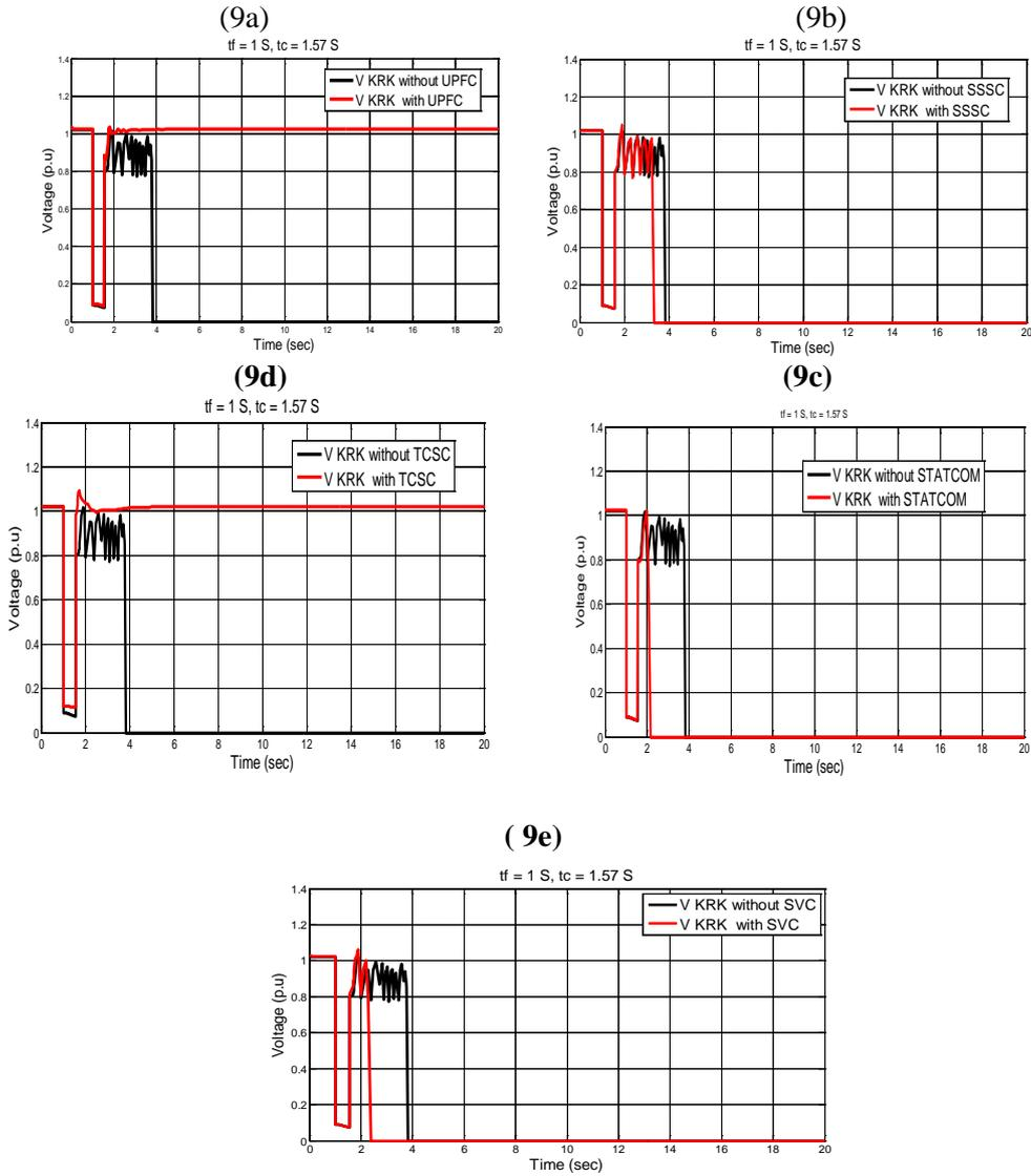
**Figure (9 a,b,c,d,e) Voltage with and without UPFC,SSSC,SVC,TCSC,STATCOM.**
