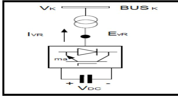
**Figure (3) STATCOM Configuration**
