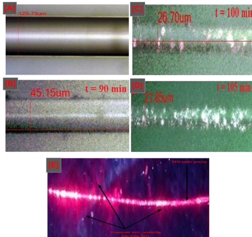
**Figure (6) the monitoring etching method by light microscope, the diameter change with etching time, realize the evanescent light around core fiber as; [A] 125  $\mu\text{m}$ , [B] 45.15  $\mu\text{m}$ , [C] 26.70  $\mu\text{m}$ , [D] 21.85  $\mu\text{m}$  and [E] evanescent light.**
