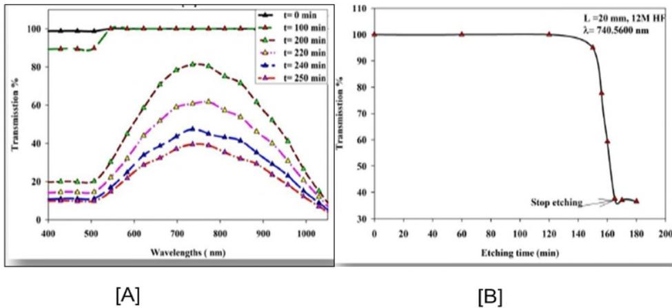
**Figure (3) [A] the transmission percentage power in fiber optics segment vs. etching time ( minute) using 12M HF solution, and [B] the transmission for  $\lambda = 740$  nm vs. Etching time (minute).**
