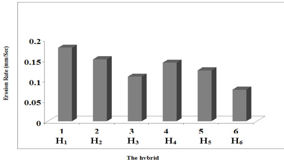
Figure (1) Systematic diagram illustrating different extents for erosion rate of prepared hybrids composites.
