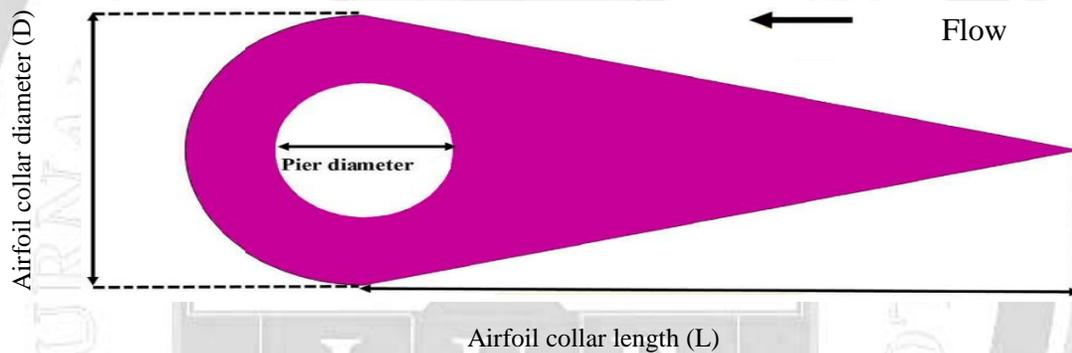
**Fig. 5: Airfoil collar shaped [38].**
