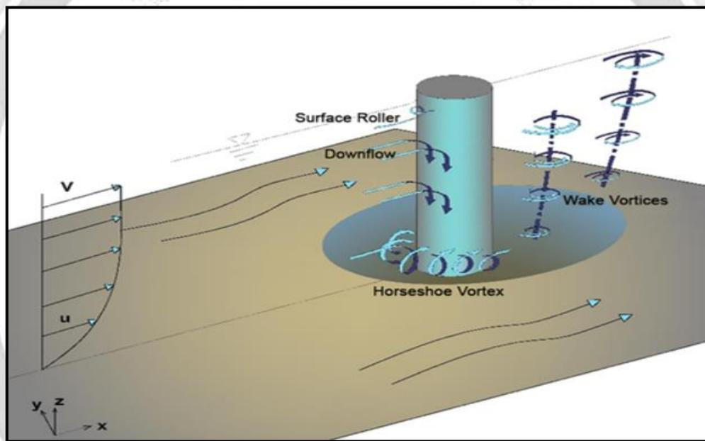
Fig. 1: Flow structure around a cylindrical bridge pier [13].
