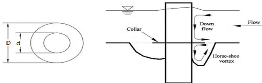
**Fig. 2: The impact of collar on pier [2].**
