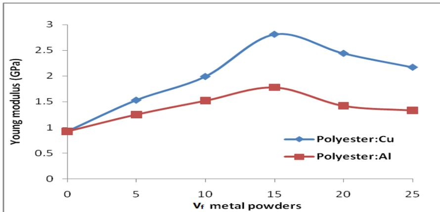
Figure (8) Young modulus of polyester composites as a function of metal powder (Cu and Al) content in composites.
