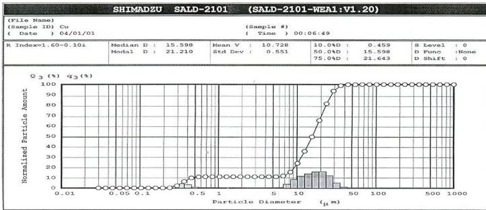
**Figure (4) Particle size analysis of Cu powder.**
