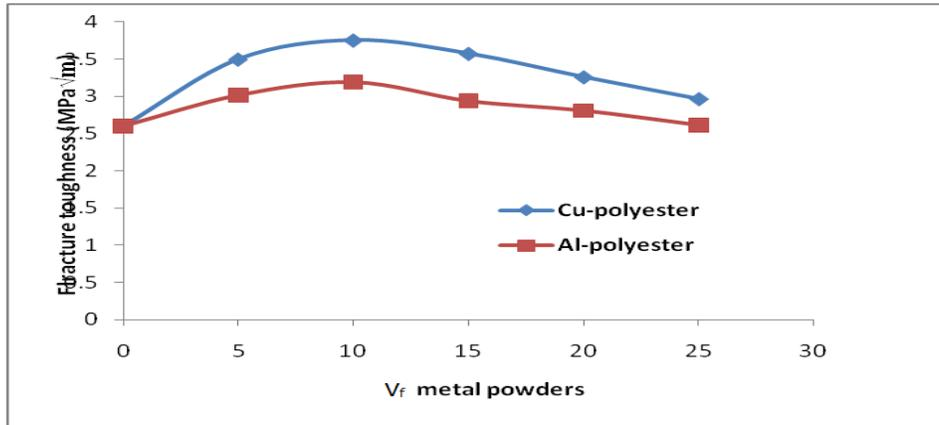
Figure (13) Fracture toughness of polyester composites as a function of metal powders content in composite.
