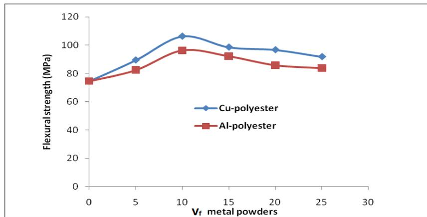
Figure (10) The flexural strength of polyester composites as a function of a metal powders content in composites.
