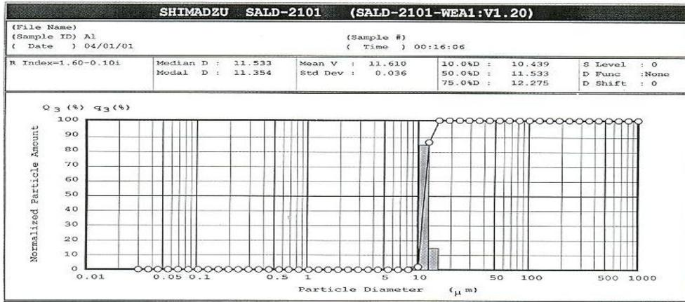
**Figure (3) Particle size analysis of Al powder.**
