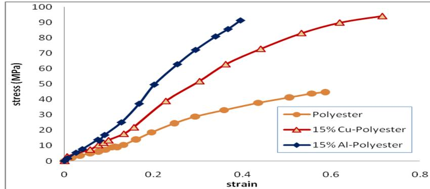
Figure (6) The (stress-strain) of unsaturated polyester and composites reinforced with the same ratio (15%  $V_f$ ) of Al and Cu.
