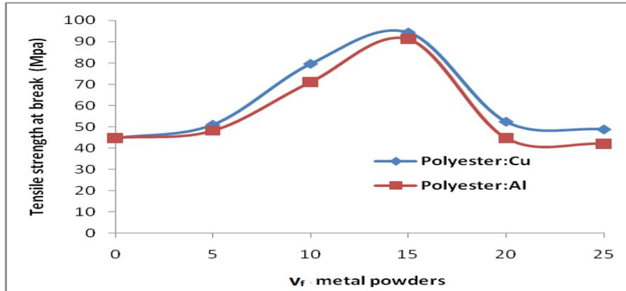
Figure (7) Tensile strength at break of polyester composites as a function of metal powders (Cu and Al) content in composites.
