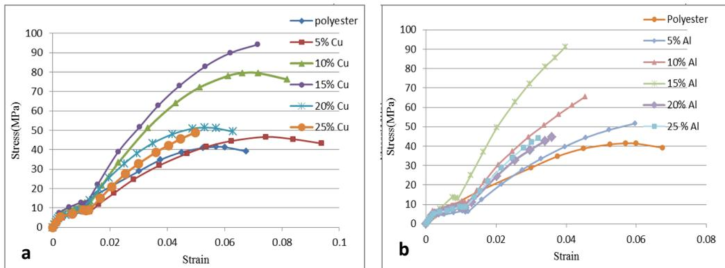
Figure(5) The stress-strain curves of unsaturated polyester composites as function of particles content in the composite (a) of Cu and (b) of Al.
