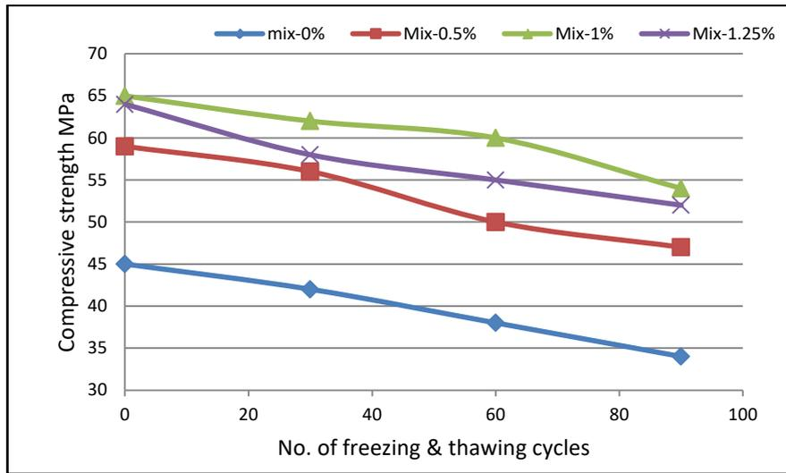
**Figure (3):- Compressive strength vs. No. of freezing and thawing cycles**
