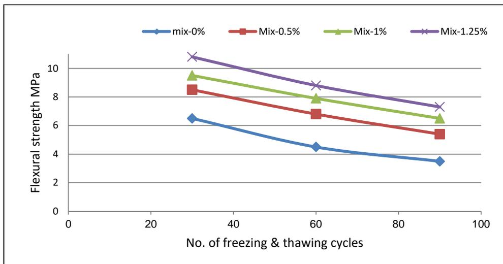
**Figure (4):- Flexural strength vs. No. of freezing and thawing cycle**
