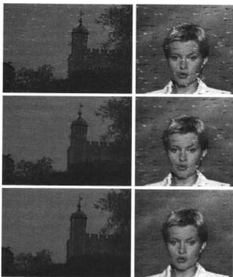
Figure 4. A frame from the original sequence (top), an output of a median filter (middle), an output of a filter with prediction error processing (bottom).
