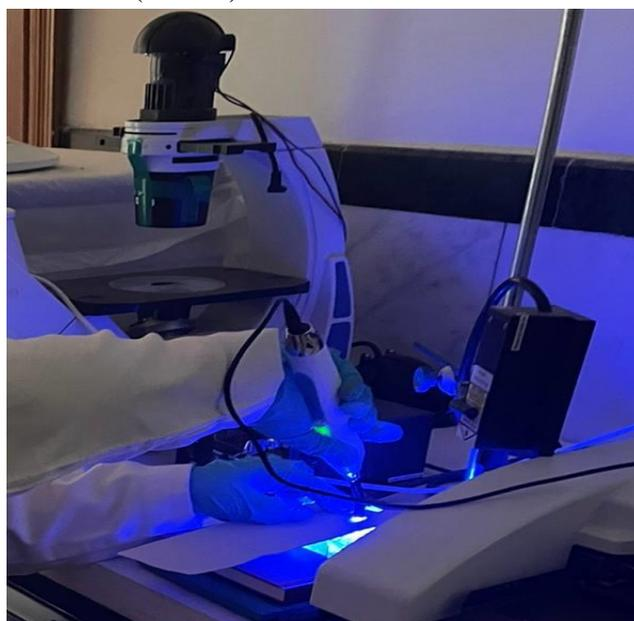
**Figure 1: Setup of Photodynamic Therapy (PDT) by blue Light emitting diode at 400  $\text{mW/cm}^2$  in this work.**
