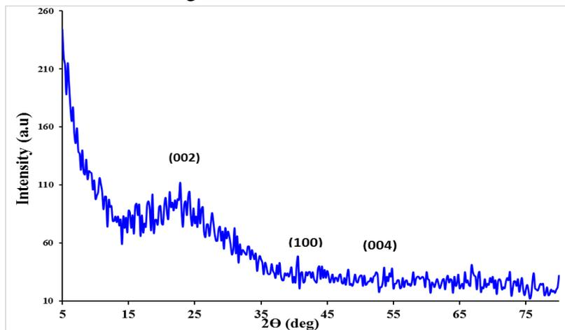
Figure 8: The XRD analysis of sample of SWCNTS-OH.
