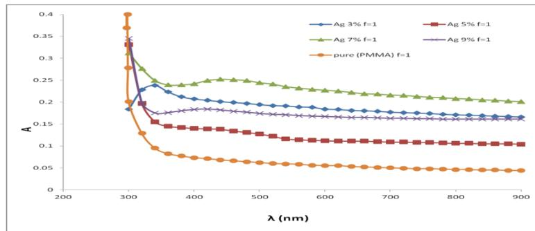
Figure (3) Absorption spectrum for pure PMMA. Ag/PMMA nanocomposite with 3,5,7, and 9wt% silver NPs.
