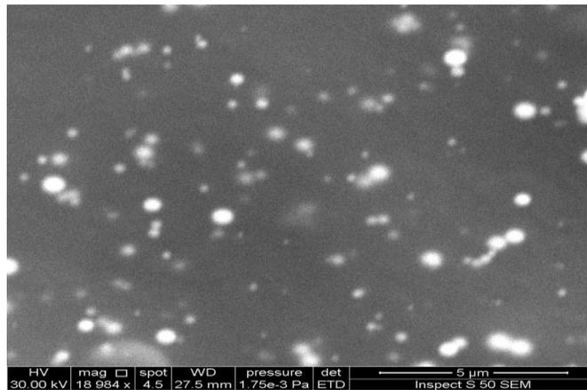
**Figure (10) SEM image for Ag/PMMA nanocomposite thin film at 5wt% silver NPs concentration.**
