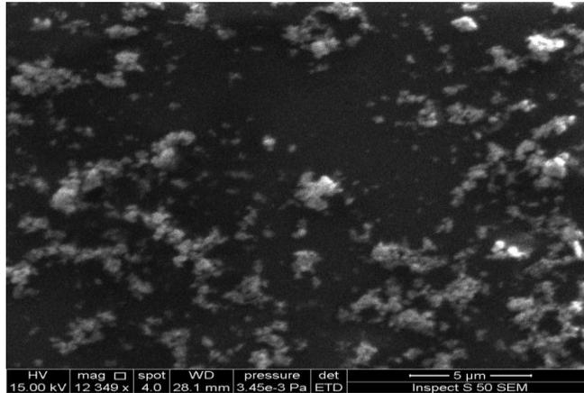
**Figure (9) SEM image for Ag/PMMA nanocomposite thin film at 9wt% silver NPs concentration.**
