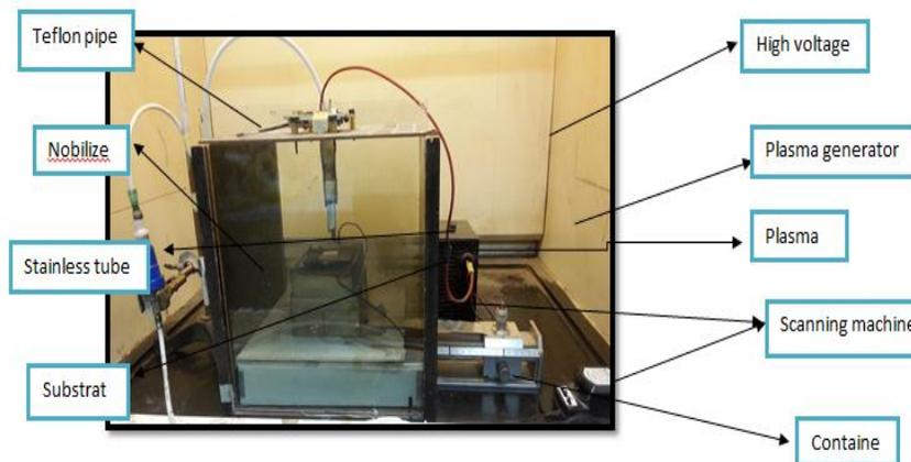
**Figure (2) Photograph for the non-equilibrium atmospheric pressure plasma system for Silver/PMMA nanocomposite thin films preparations.**
