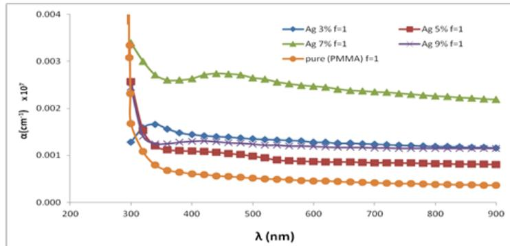
Figure (4) Absorption coefficient for pure PMMA, Ag/PMMA nanocomposite with 3,5,7 and 9wt% silver NPs.
