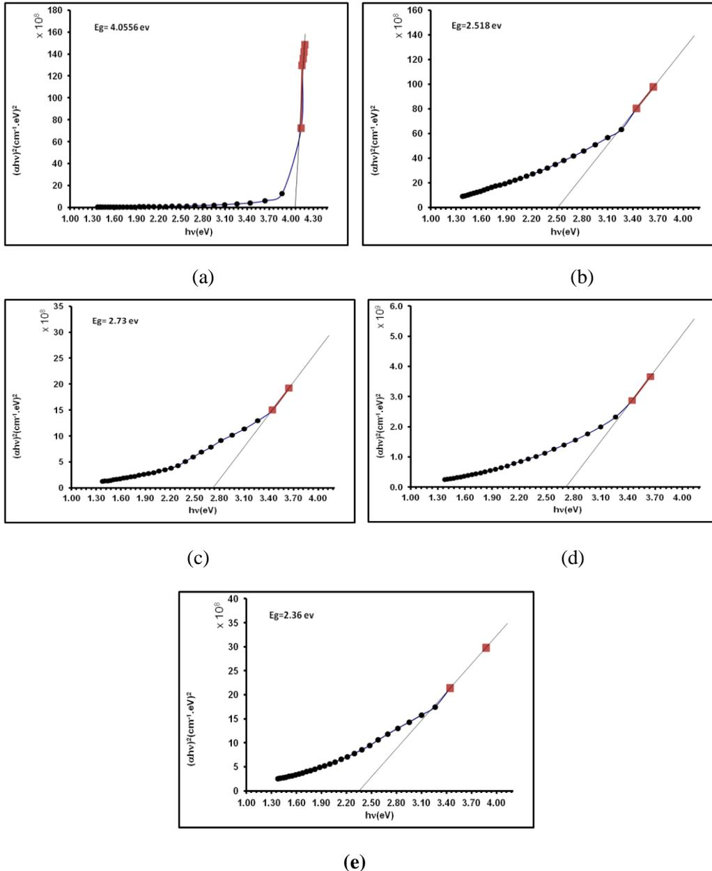
**Figure (5) The  $E_g$  for (a) pure PMMA film, (b) 3wt% silver concentration, (c) 5wt%, (d) 7wt% and (e) 9wt%. all at constant gas flow rate 1L/min.**
