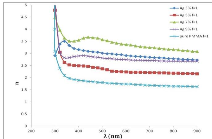
**Figure (6)**The variation of the refractive index (n) with wavelength for pure PMMA Ag/PMMA nanocomposite with 3,5,7,9 wt% silver NPs.
