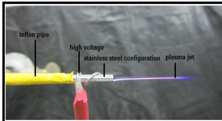
**Figure (1) Photograph at working of the non-thermal atmospheric pressure plasma torch.**
